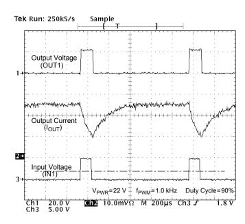
Figure 11. Output Voltage and Output Current vs. Input Voltage at V<sub>PWR</sub>=22 V, PMW Frequency of 1.0 kHz, and Duty Cycle of 90%
