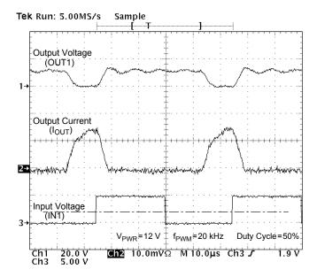
Figure 14. Output Voltage and Output Current vs. Input Voltage at V<sub>PWR</sub>=12 V, PMW Frequency of 20 kHz, and Duty Cycle of 50% for a Purely Resistive Load
