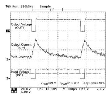
Figure 8. Output Voltage and Output Current vs. Input Voltage at V<sub>PWR</sub>=24 V, PMW Frequency of 1.0 kHz, and Duty Cycle of 10%
