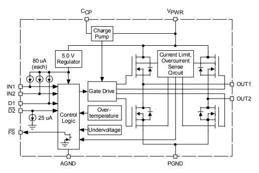
Figure 1. 33886 Internal Block Diagram
