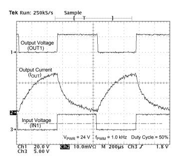
Figure 9. Output Voltage and Output Current vs. Input Voltage at V<sub>PWR</sub>=24 V, PMW Frequency of 1.0 kHz, and Duty Cycle of 50%
