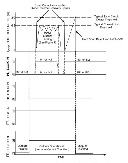
Figure 6. Output Load Current Limiting Versus Time
