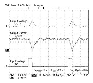
Figure 15. Output Voltage and Output Current vs. Input Voltage at  $V_{PWR}$ =12 V, PMW Frequency of 20 kHz, and Duty Cycle of 90% for a Purely Resistive Load
