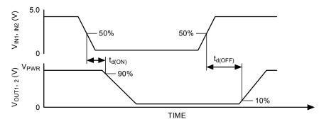
Figure 2. Output Delay Time
