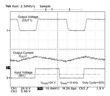
Figure 12. Output Voltage and Output Current vs. Input Voltage at V<sub>PWR</sub>=24 V, PMW Frequency of 10 kHz, and Duty Cycle of 50%
