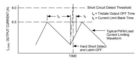
Figure 7. PWM Current Limiting Detail
