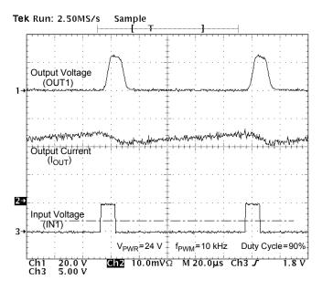
Figure 13. Output Voltage and Output Current vs. Input Voltage at V<sub>PWR</sub>=24 V, PMW Frequency of 10 kHz, and Duty Cycle of 90%
