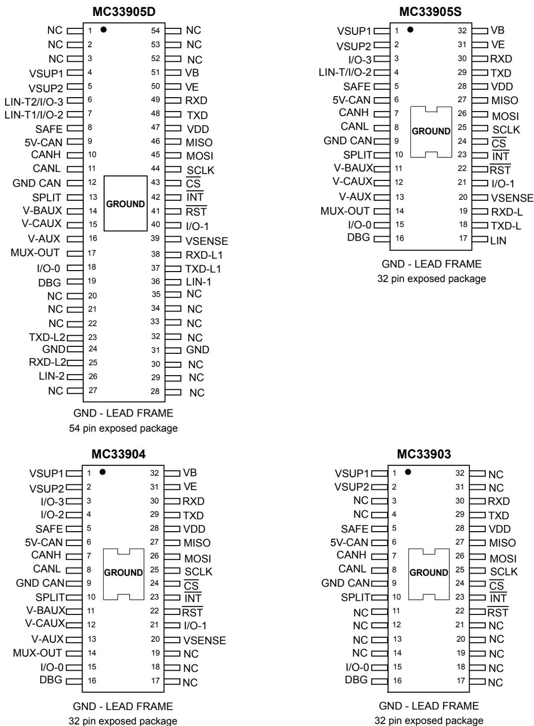
Note: MC33905D, MC33905S, MC33904 and MC33903 are footprint compatible,
