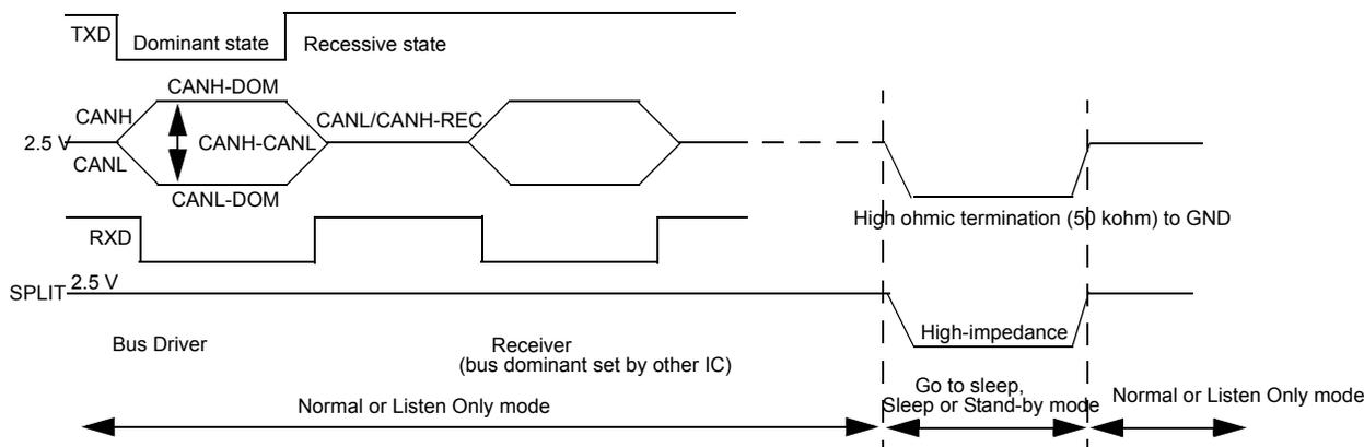
Figure 34. Bus signal in TXD/RXD and LP mode
