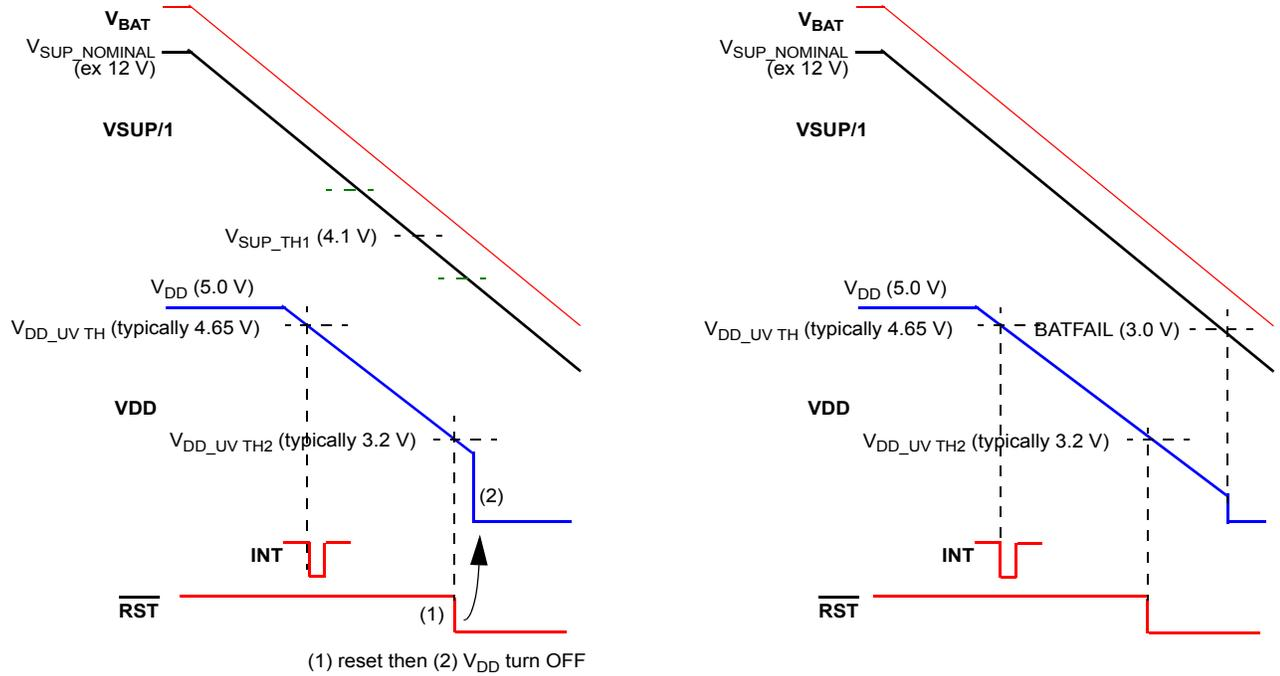
Case 5: “ $V_{DD\_UV\_TH}$  3.2V”, with bit Crank = 0 (default value)
