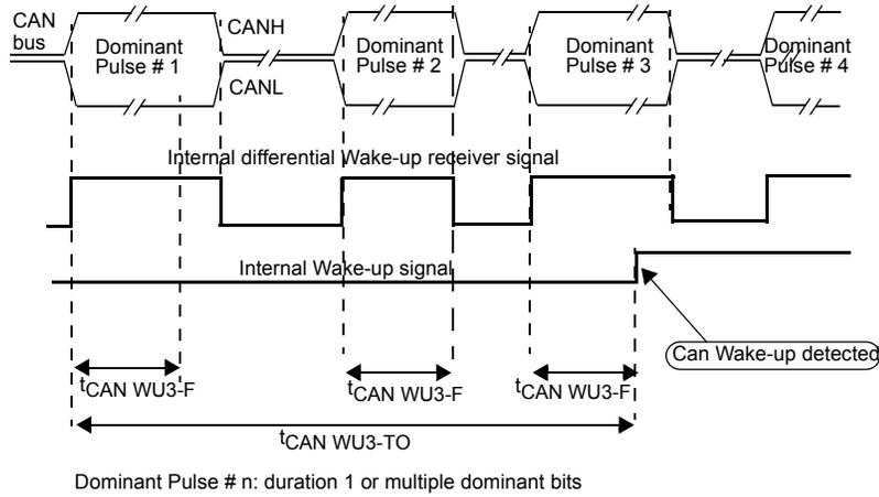
Figure 36. Pattern wake-up - multiple dominant detection
