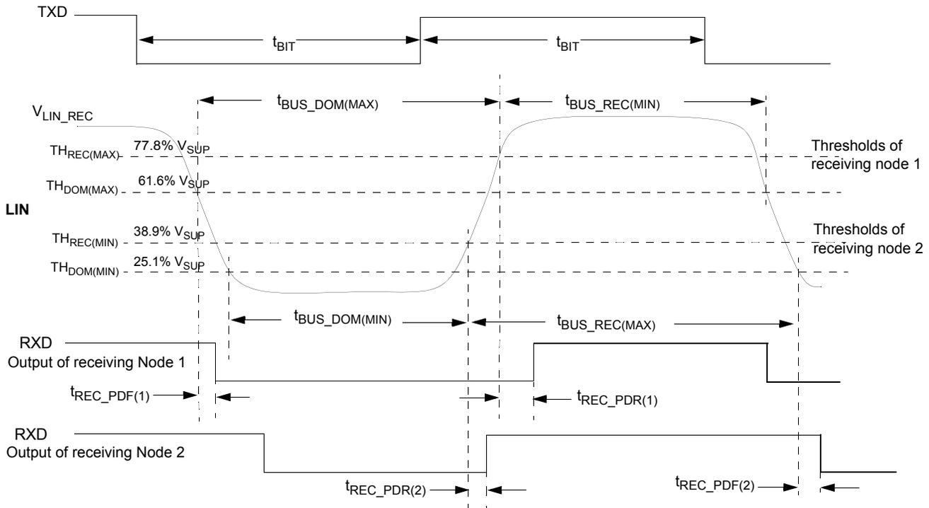
Figure 19. LIN timing measurements for slow slew rate
