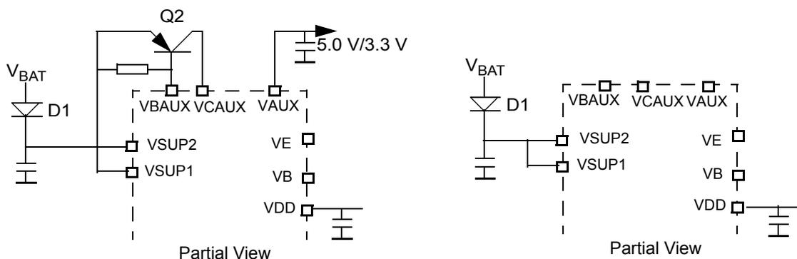
ex 3: No External Transistor, V<sub>DD</sub> ~100 mA Capability delivered by internal path transistor.
