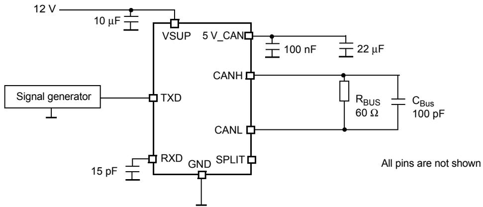
Figure 17. Test circuit for CAN timing characteristics
