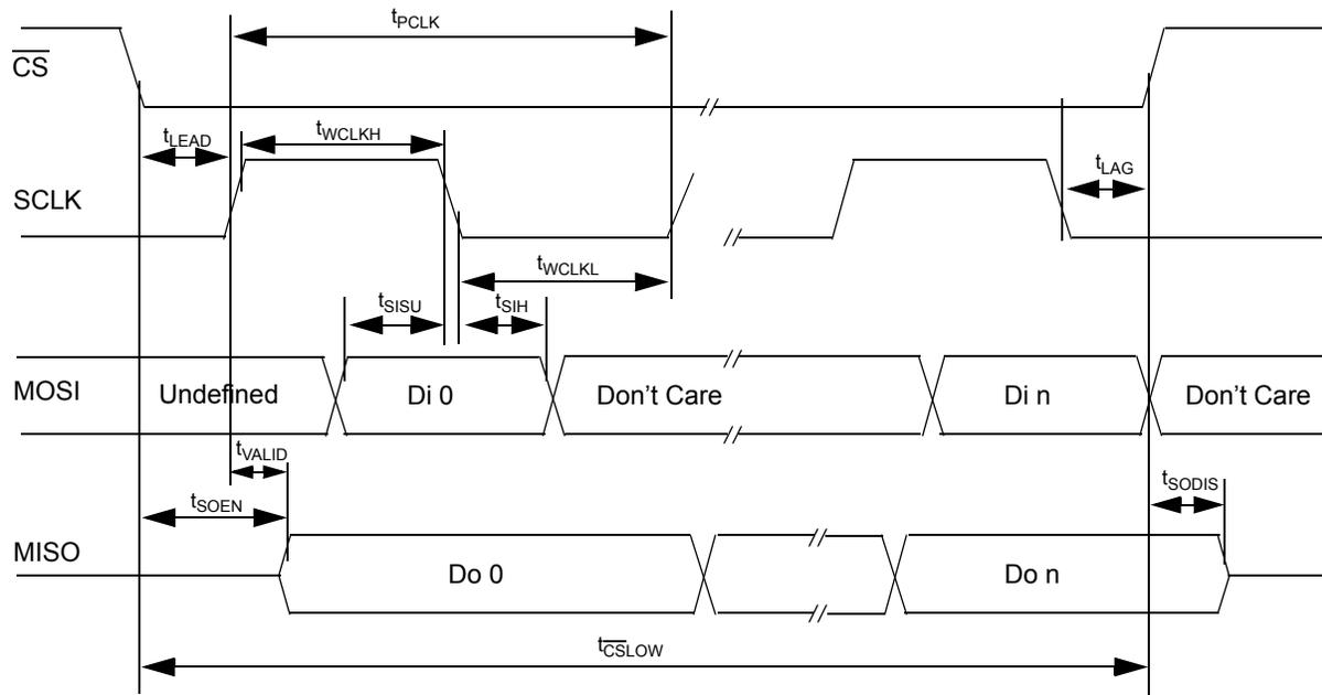
Figure 14. SPI timing
