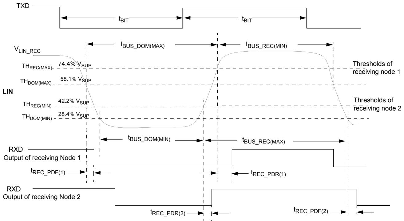
Figure 18. LIN timing measurements for normal slew rate
