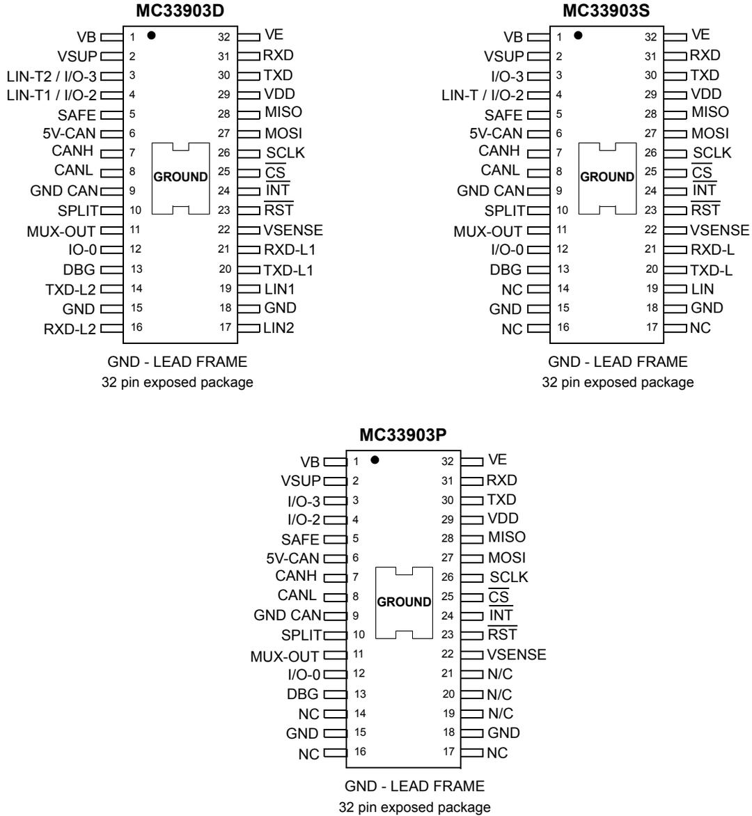
Note: MC33903D, MC33903S, and MC33903P are footprint compatible.
