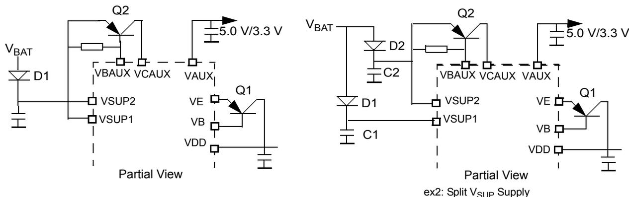
Optimized solution for cranking pulses.
