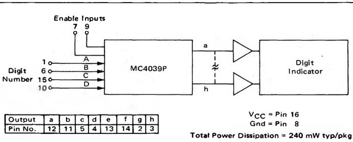
The MC4039P is derived from the XC170 128-Bit Read Only Memory. It can directly operate low-voltage lamp indicators. A four digit binary input is translated into combinations of the eight outputs. These combinations correspond to different illuminated segments of the seven-bar digit indicator. The input and output codes with their related numerical digits are shown in the diagram. The enable inputs can be used for automatic blanking.
