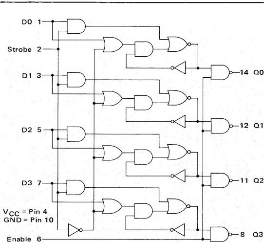
This monolithic device consists of four latch circuits with open collector outputs, common Strobe input, and output enable input. The output of each latch will follow the data input when the Strobe input is in a logical "1" state. When the Strobe is in a logical "0" state, the latch will store the logic state of the data input just prior to the change of the Strobe from a "1" level to a "0" level.
