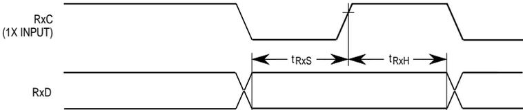
Figure 5-9. Receiver Timing
