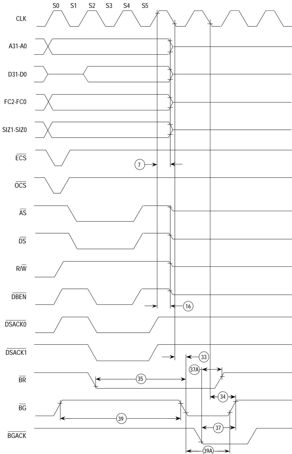
NOTE: Timing measurements are referenced to and from a low voltage of 0.8 V and a high voltage of 2.0 V, unless otherwise noted. The voltage swing through this range should start outside and pass through the range so that the rise or fall will be linear between 0.8 V and 2.0 V.
