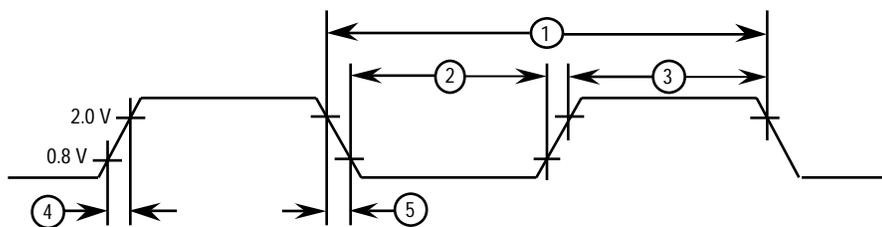
NOTE: Timing measurements are referenced to and from a low voltage of 0.8 V and a high voltage of 2.0 V, unless otherwise noted. The voltage swing through this range should start outside and pass through the range so that the rise or fall will be linear between 0.8 V and 2.0 V.
