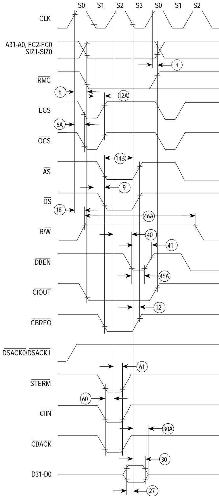
Figure 13. Synchronous Read Cycle Timing Diagram
