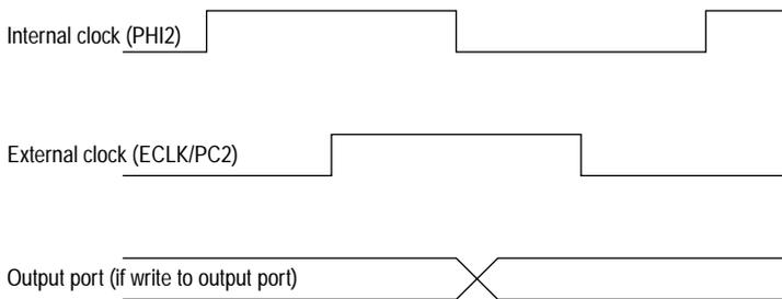
**Figure 4-2** ECLK timing diagram
