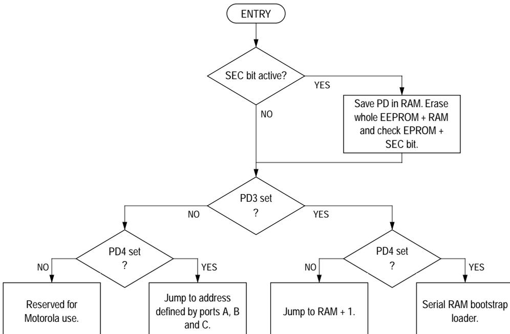
**Figure 2-1** Bootstrap mode function selection flow chart
