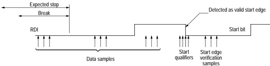
**Figure 7-7** SCI start bit following a break
