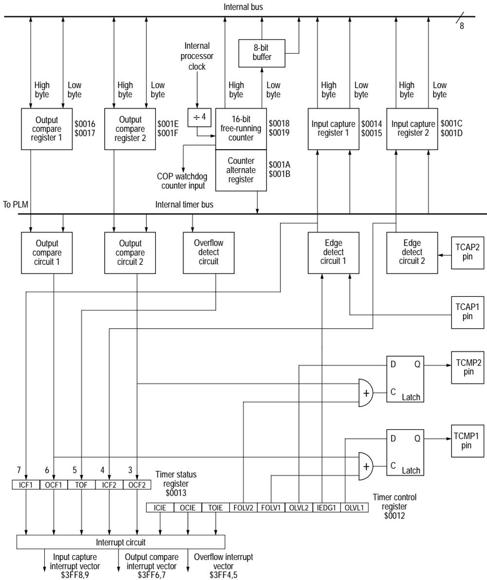
Figure 6-1 16-bit programmable timer block diagram
