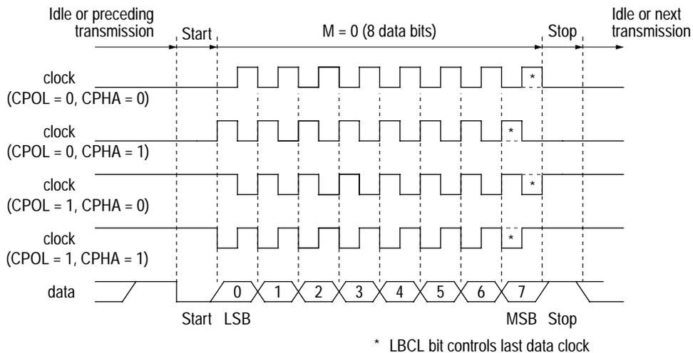
**Figure 7-9** SCI data clock timing diagram (M=0)
