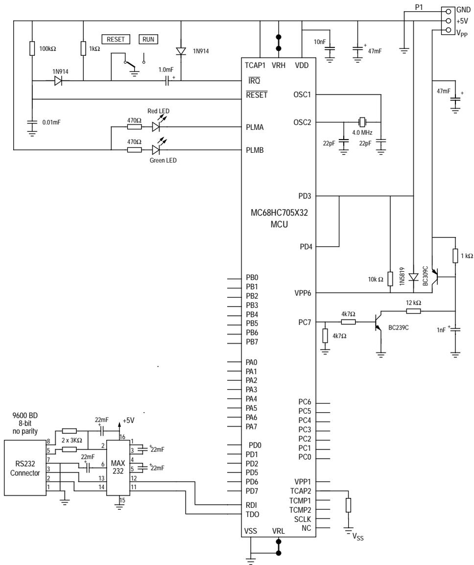
Figure B-7 RAM load and execute schematic diagram
