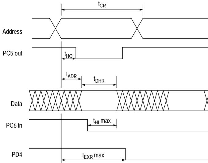
**Figure B-8** Parallel RAM loader timing diagram
