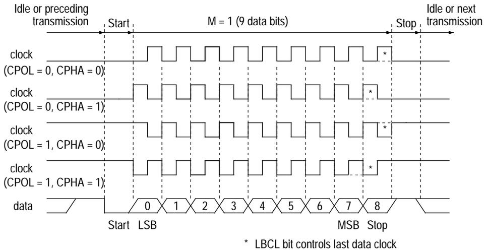
**Figure 7-10** SCI data clock timing diagram (M=1)
