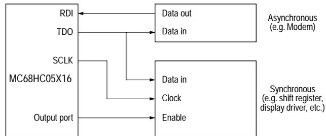
**Figure 7-8** SCI example of synchronous and asynchronous transmission
