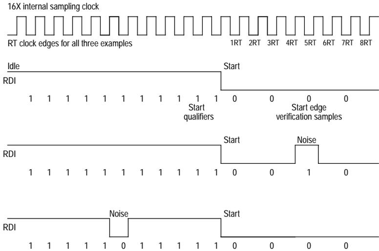
**Figure 7-4** SCI examples of start bit sampling technique
