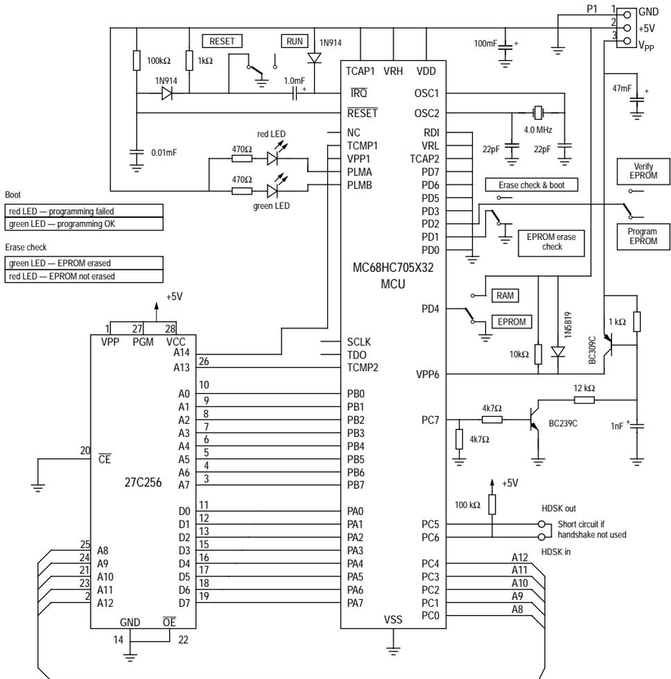
**Figure B-6** EPROM parallel bootstrap schematic diagram
