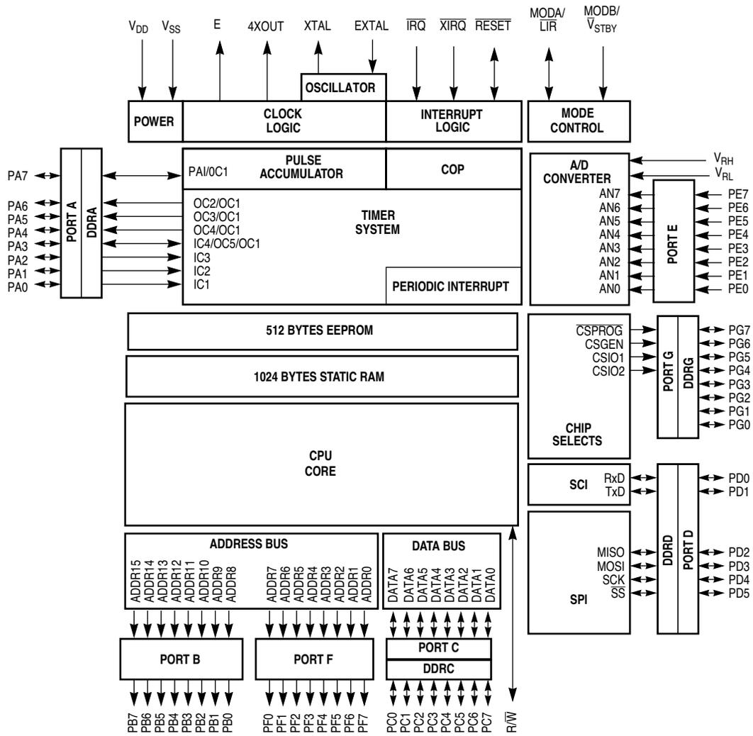
Figure 1 MC68HC11F1 Block Diagram
