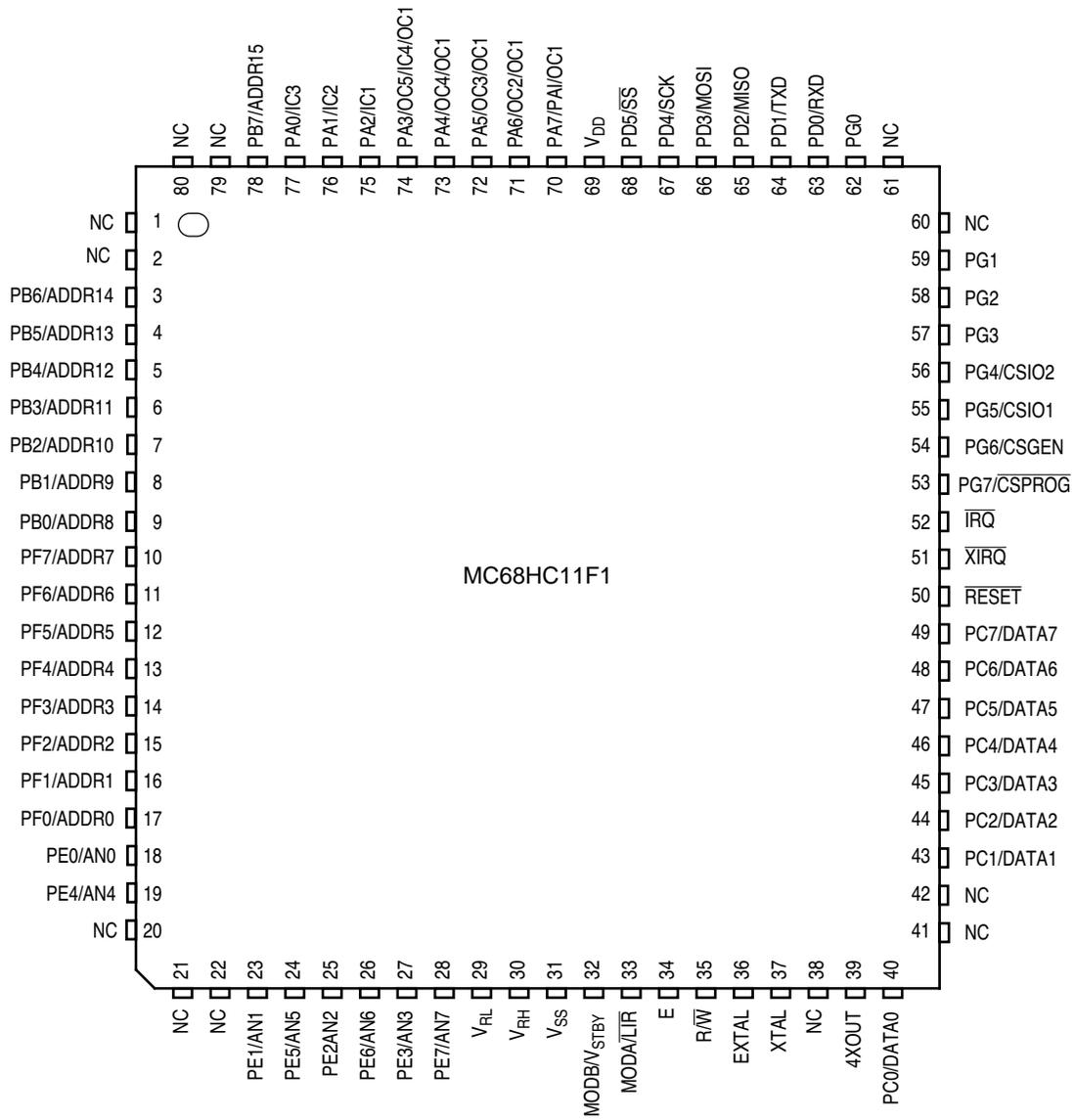
**Figure 4 Pin Assignments for the MC68HC11F1 80-Pin QFP**
