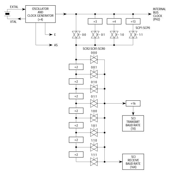
Figure 8 SCI Baud Rate
