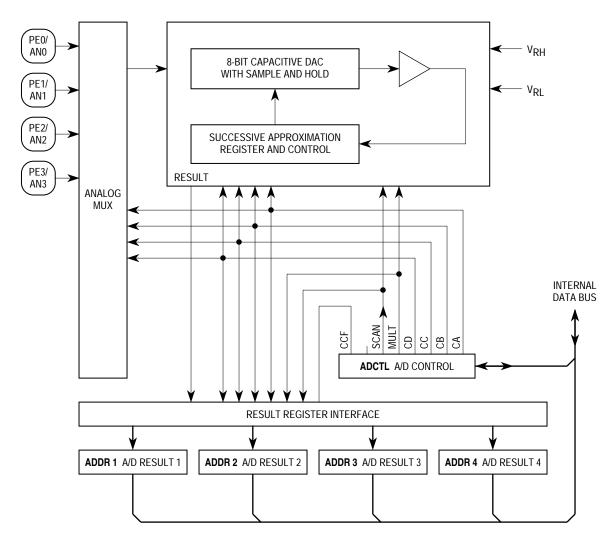
Figure 13 A/D Converter Block Diagram
