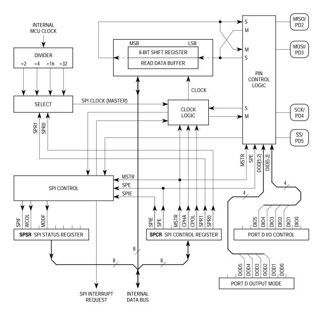
Figure 9 SPI Block Diagram
