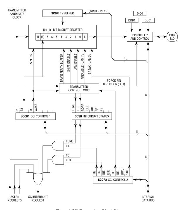
Figure 6 SCI Transmitter Block Diagram
