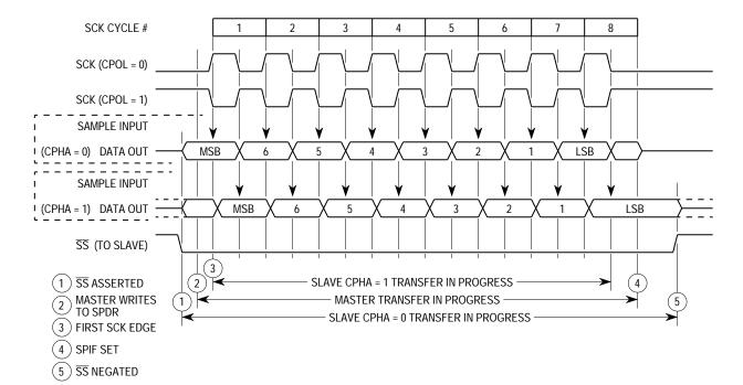
Figure 10 SPI Transfer Format
