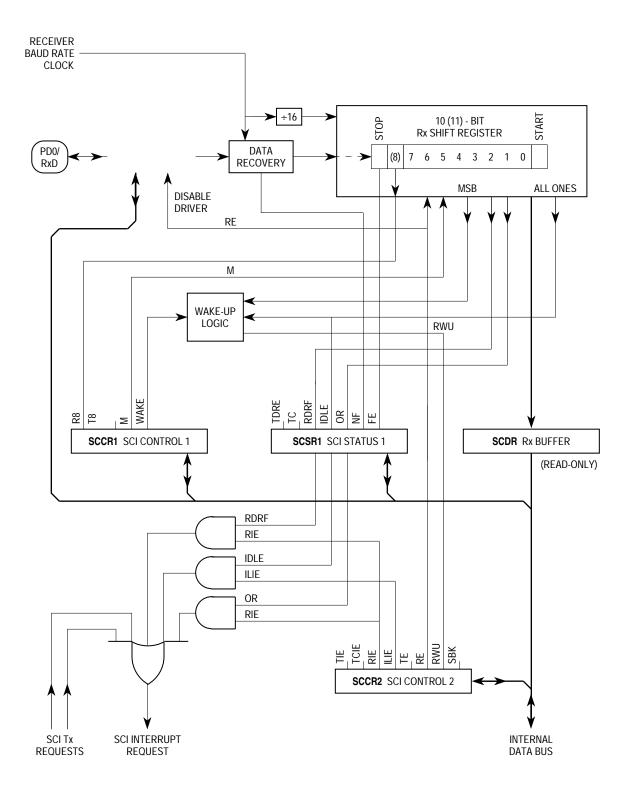
Figure 7 SCI Receiver Block Diagram
