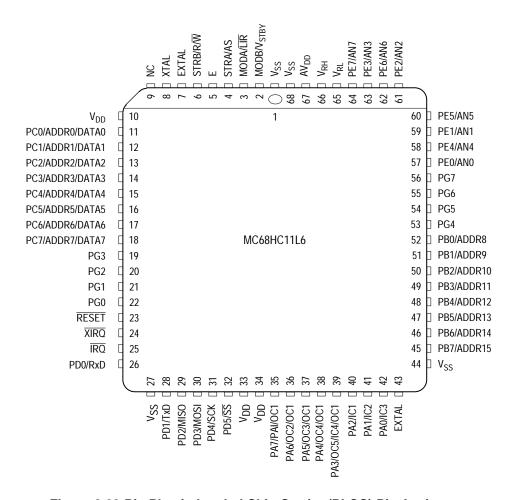
Figure 2 68-Pin Plastic-Leaded Chip Carrier (PLCC) Pin Assignments
