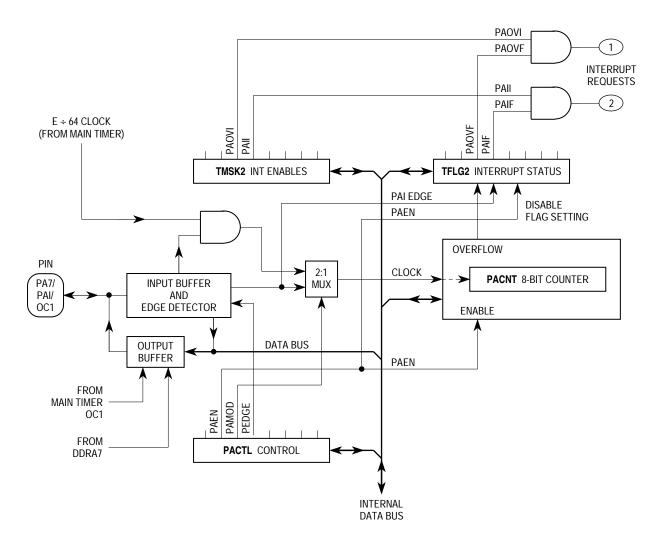
Figure 12 Pulse Accumulator System Block Diagram
