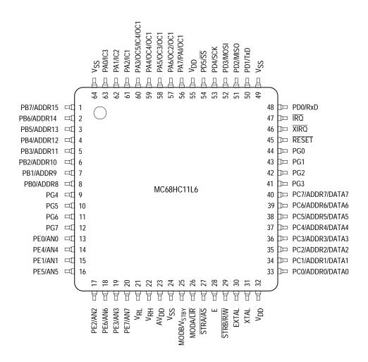
Figure 1 64-Pin Quad Flat Pack (QFP) Pin Assignments
