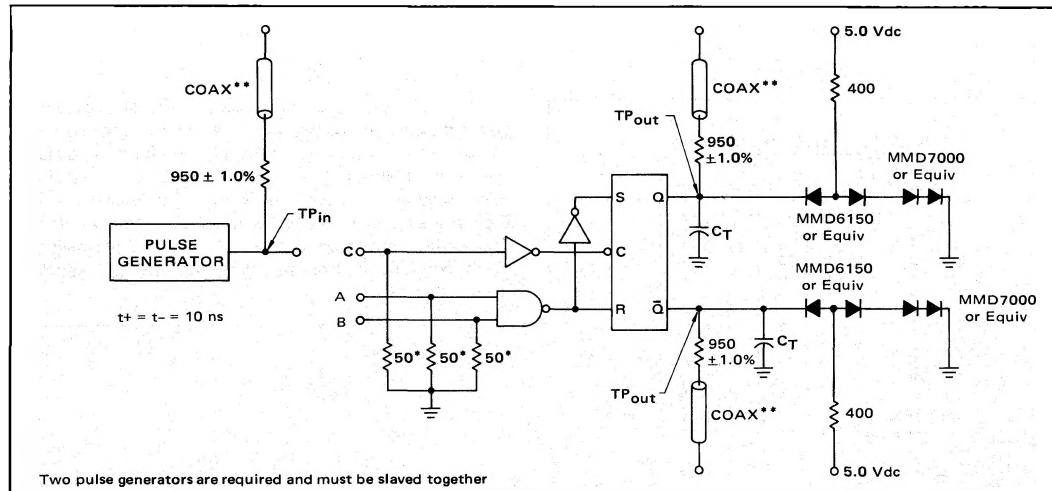
Two pulse generators are required and must be slaved together to provide the waveforms shown. Pulse generator for Pulses A and B must be operated in the double pulse mode.
