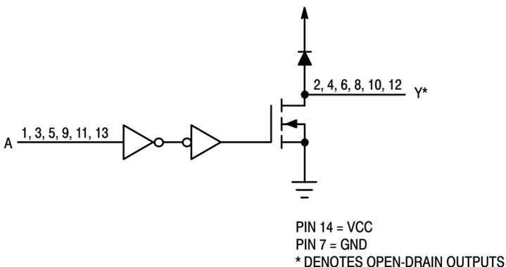
Figure 2. Logic Diagram
