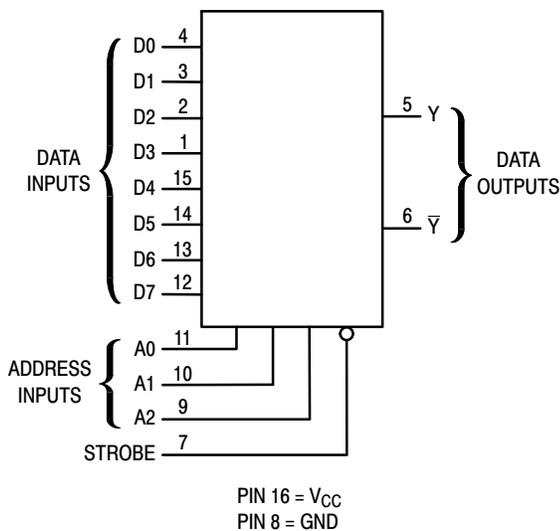
Figure 1. Logic Diagram
