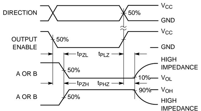
Figure 2. Switching Waveform
