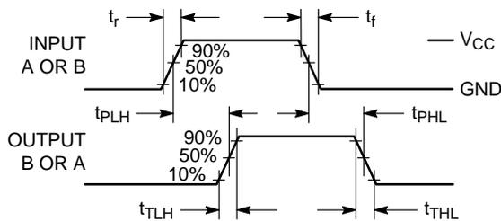
Figure 1. Switching Waveform
