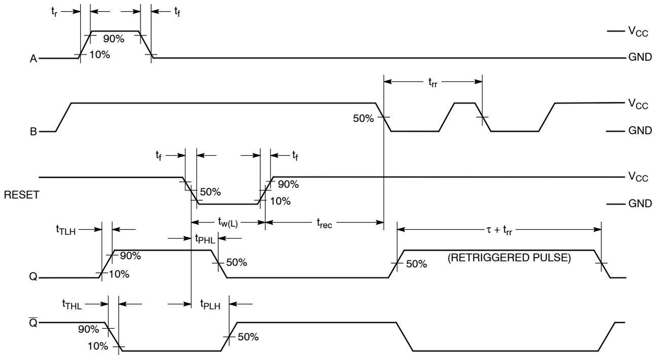
**Figure 9. Switching Waveform**
