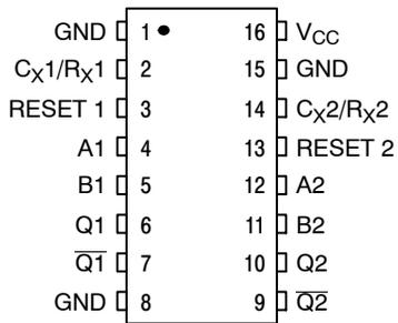
Figure 1. Pin Assignment
