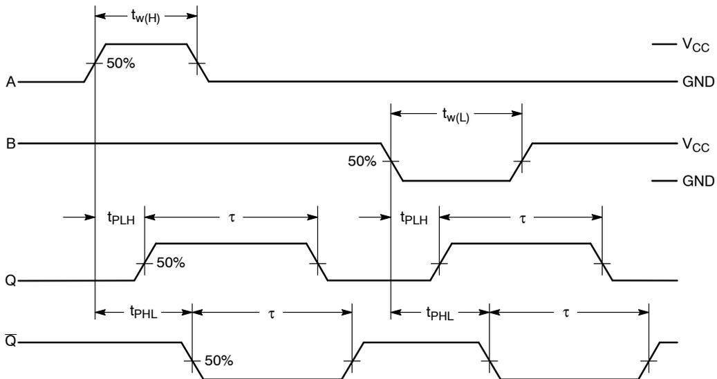
**Figure 8. Switching Waveform**
