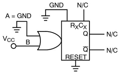
Figure 16. Connection of Unused Section
