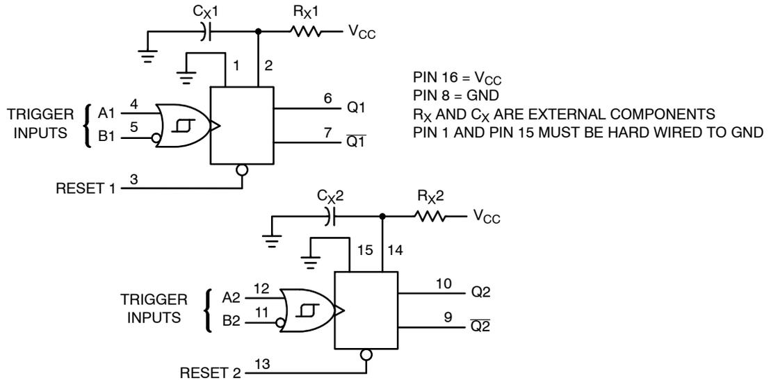
Figure 2. Logic Diagram
