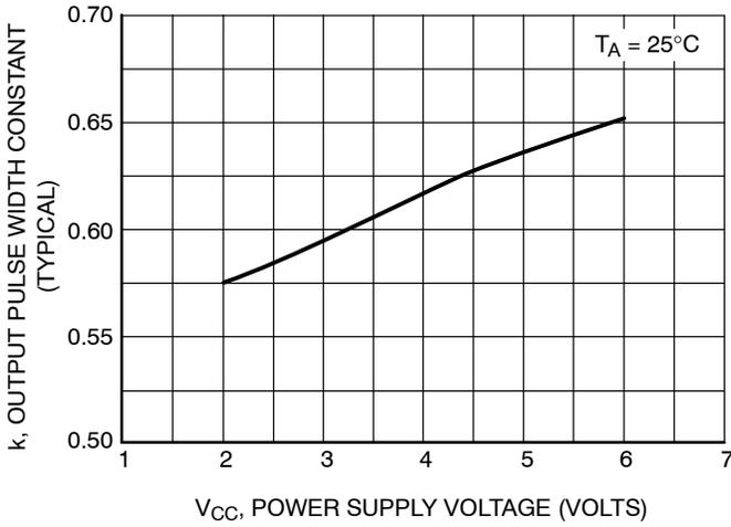
**Figure 3. Typical Output Pulse Width Constant, k, versus Supply Voltage**
