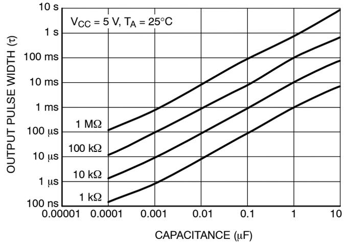
**Figure 4. Output Pulse Width versus Timing Capacitance**
