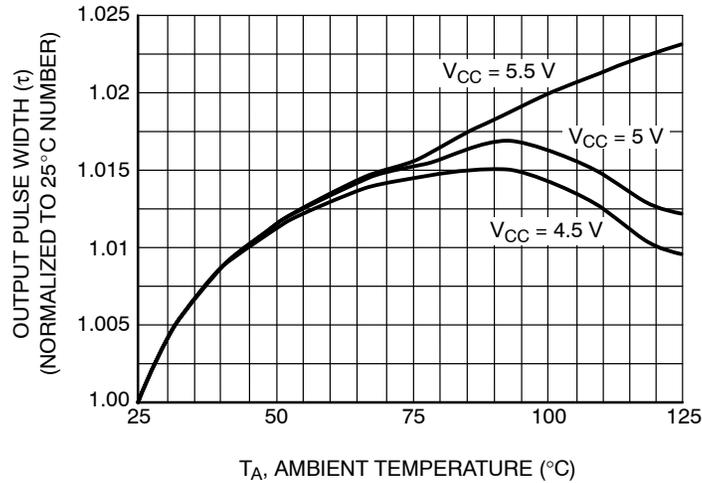
**Figure 7. Normalized Output Pulse Width versus Power Supply Voltage**
