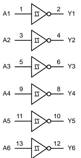
$Y = \bar{A}$       PIN 14 =  $V_{CC}$
