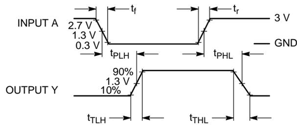
**Figure 1. Switching Waveforms**
