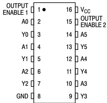
Figure 1. Pin Assignment
