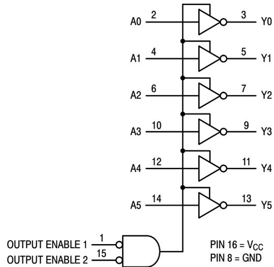
Figure 2. Logic Diagram
