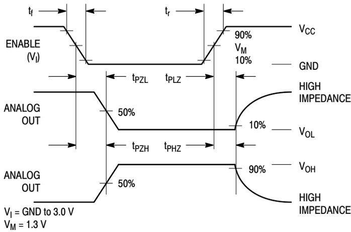
**Figure 17. Propagation Delays, Enable to Analog Out**
