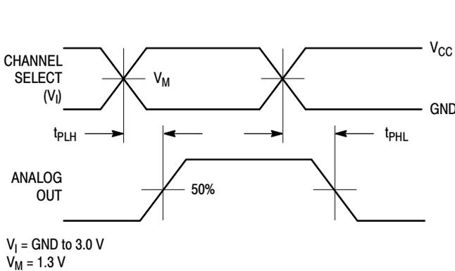
Figure 13. Propagation Delays, Channel Select to Analog Out
