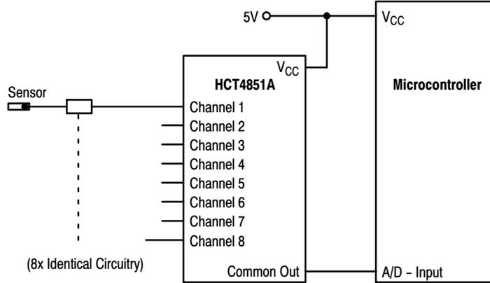
**Figure 8. MC74HCT4851A Solution**
