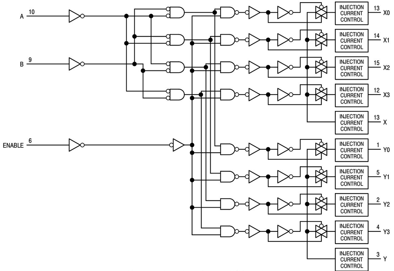
Figure 22. Function Diagram, HCT4852A
