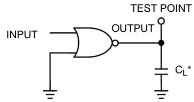
\*Includes all probe and jig capacitance
