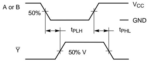
**Figure 4. Switching Waveforms**
