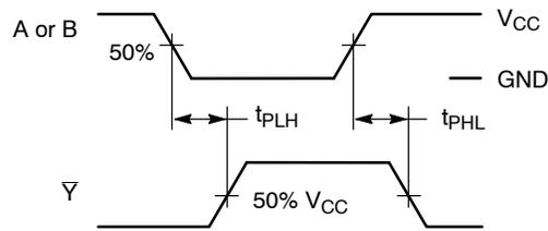
**Figure 4. Switching Waveforms**
