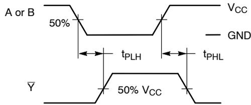
Figure 4. Switching Waveforms
