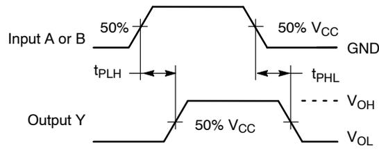
**Figure 4. Switching Waveforms**
