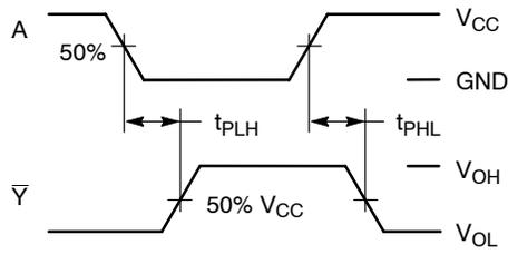
**Figure 4. Switching Waveforms**
