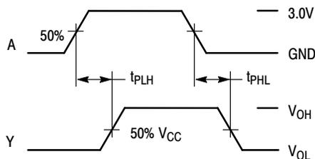
Figure 1. Switching Waveforms
