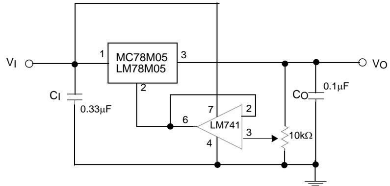
Figure 4. Adjustable Output Regulator (7 to 30V)
