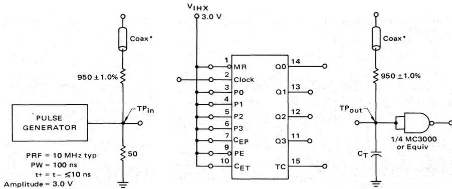
$C_T = 15$  pF = total parasitic capacitance, which includes probe, wiring, and load capacitances.
