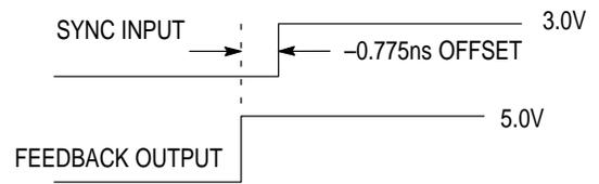
**Figure 2. Depiction of the Fixed SYNC to Feedback Offset ( $t_{PD}$ ) Which is Present When a 470KΩ Resistor is Tied to VCC or Ground**
