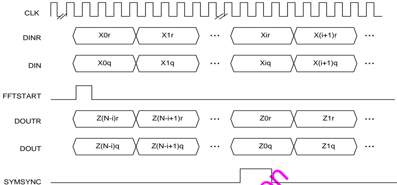
Figure 3. Data I/O for the Non-multiplexed Mode
