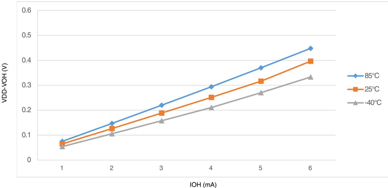
Figure 1. Typical I<sub>OH</sub> Vs. V<sub>DD</sub>-V<sub>OH</sub> (standard drive strength) (V<sub>DD</sub> = 5 V)
