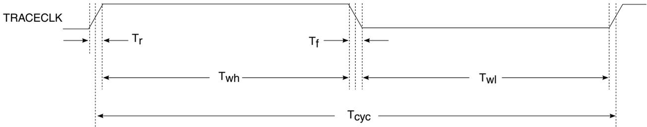
Figure 7. TRACE\_CLKOUT specifications
