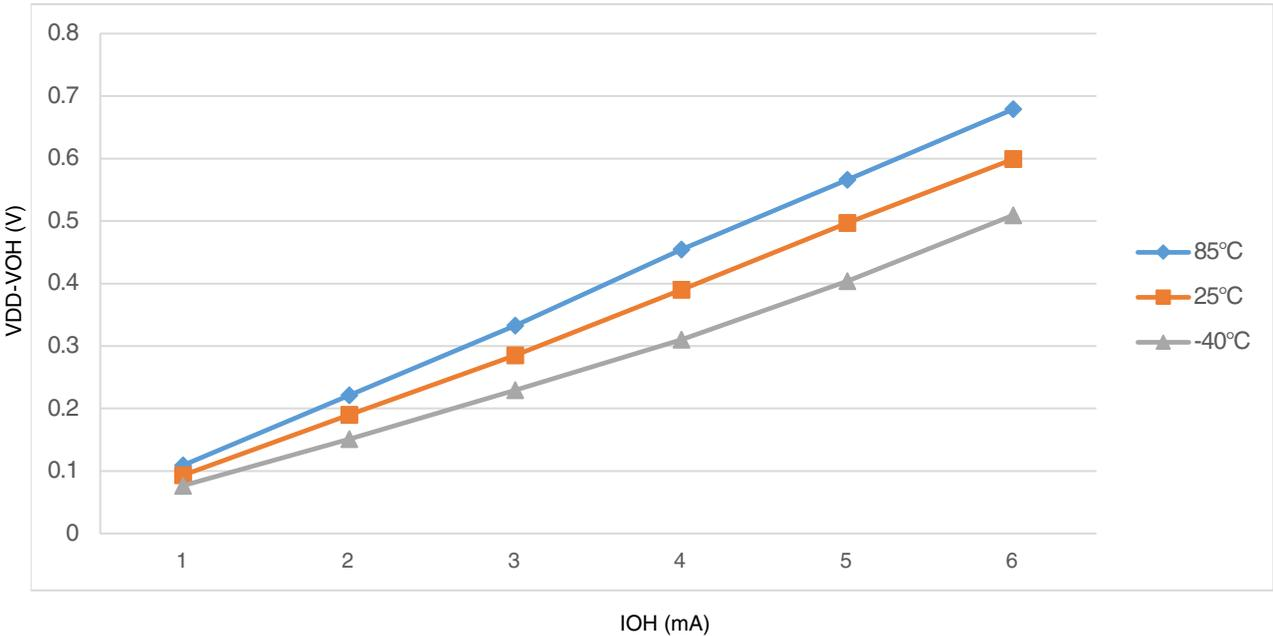
Figure 2. Typical I<sub>OH</sub> Vs. V<sub>DD</sub>-V<sub>OH</sub> (standard drive strength) (V<sub>DD</sub> = 3 V)
