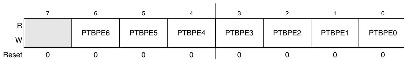
Figure 6-9. Internal Pullup Enable for Port B (PTBPE)
