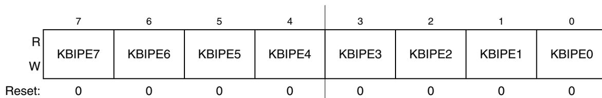
**Figure 7-4. KBI Pin Enable Register**
