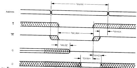
3. If the  $\overline{S}$  low transition occurs simultaneously with the  $\overline{W}$  low transition, the output buffers remain in a high-impedance state.
