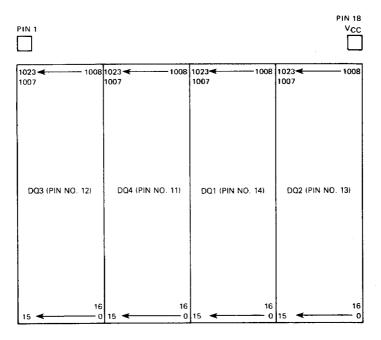
To determine the precise location on the die of a word in memory, reassign address numbers to the address pins as in the table below. The bit locations can then be determined directly from the bit map.
