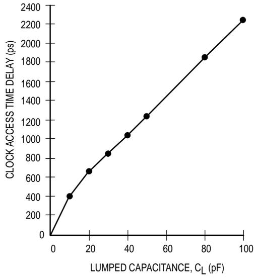
**Figure 3. Lumped Capacitive Load and Typical Derating Curve**
