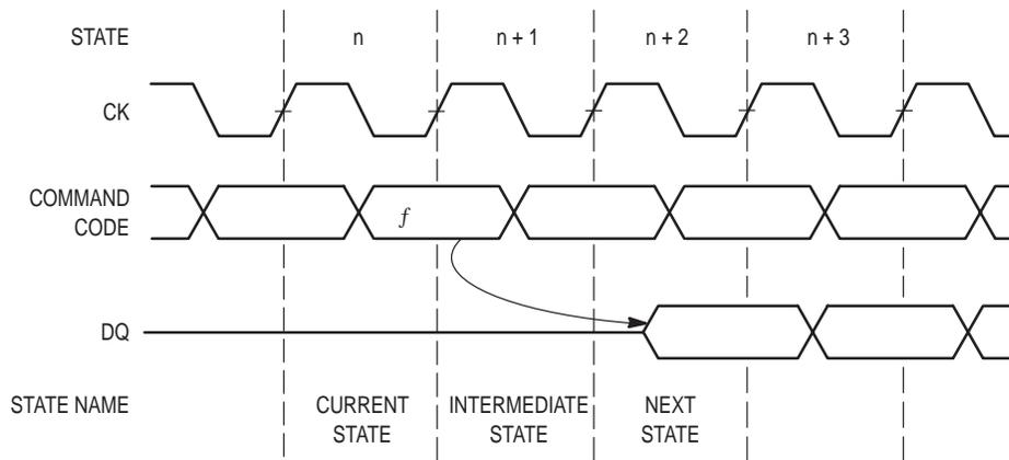
**Figure 4. State Definitions for I/O State Diagrams**
