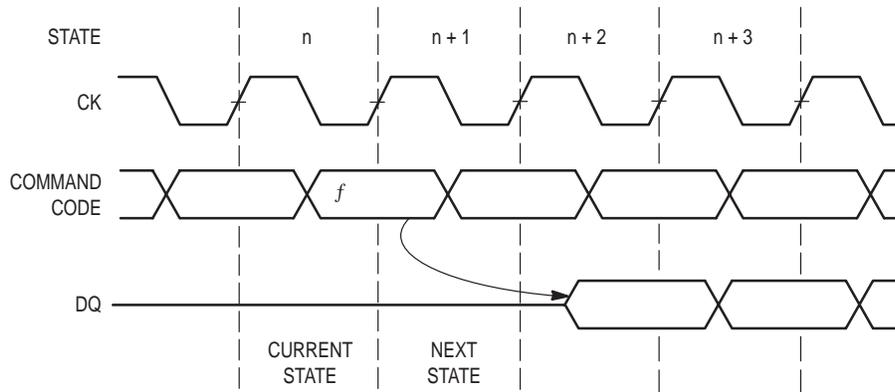
Figure 2. State Definitions for ZBT RAM State Diagram
