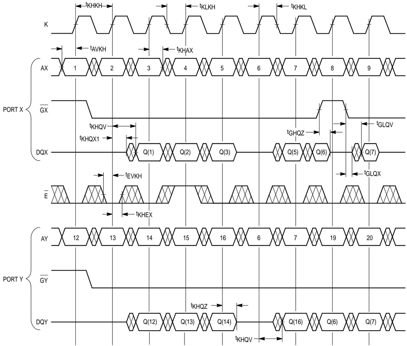
NOTE:  $\overline{E}$  Low =  $\overline{E1}$  Low and  $\overline{E2}$  High.  $\overline{E}$  High =  $\overline{E1}$  High or  $\overline{E2}$  Low.
