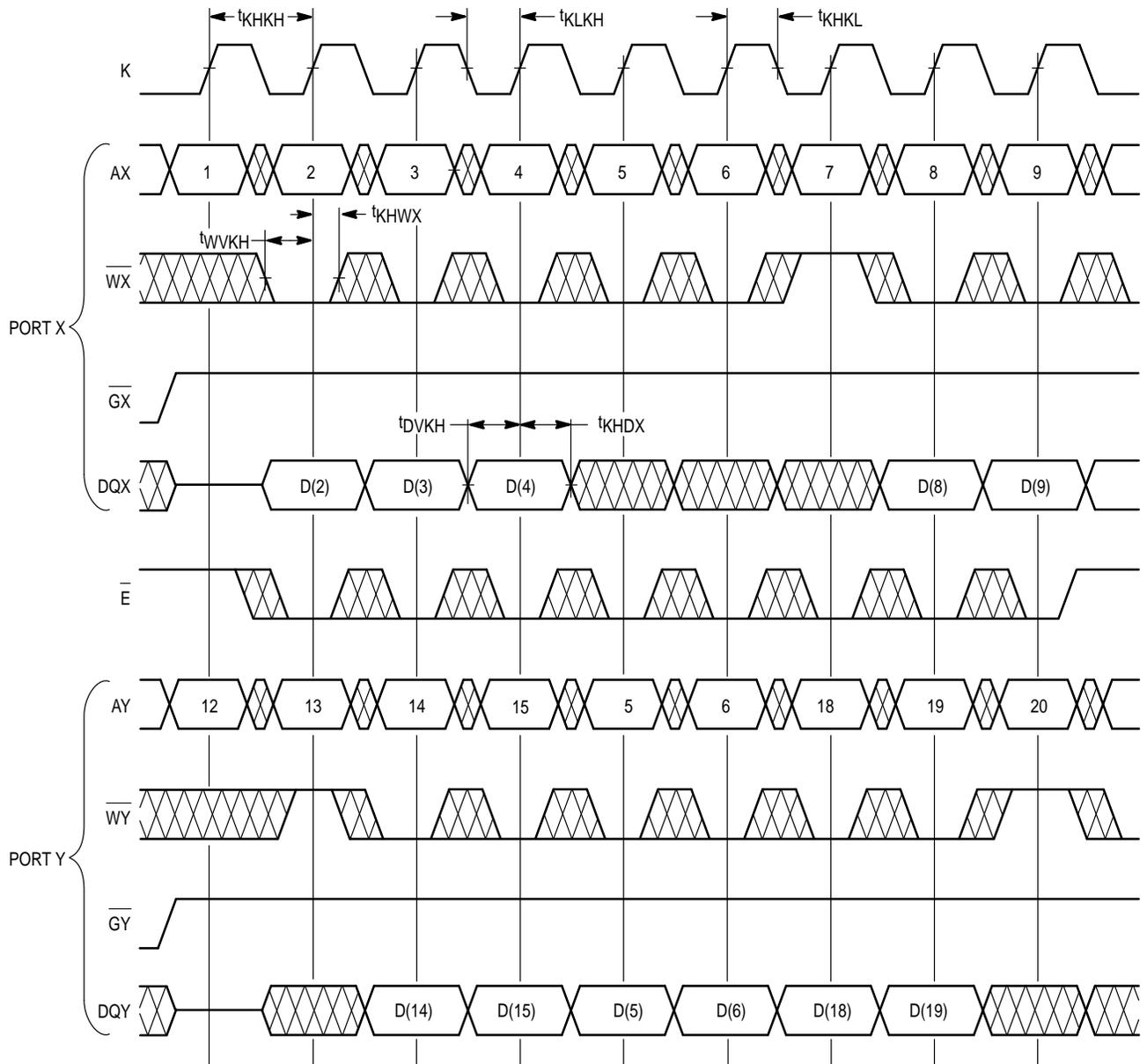
NOTE:  $\overline{E}$  Low =  $\overline{E1}$  Low and  $\overline{E2}$  High.  $\overline{E}$  High =  $\overline{E1}$  High or  $\overline{E2}$  Low.
