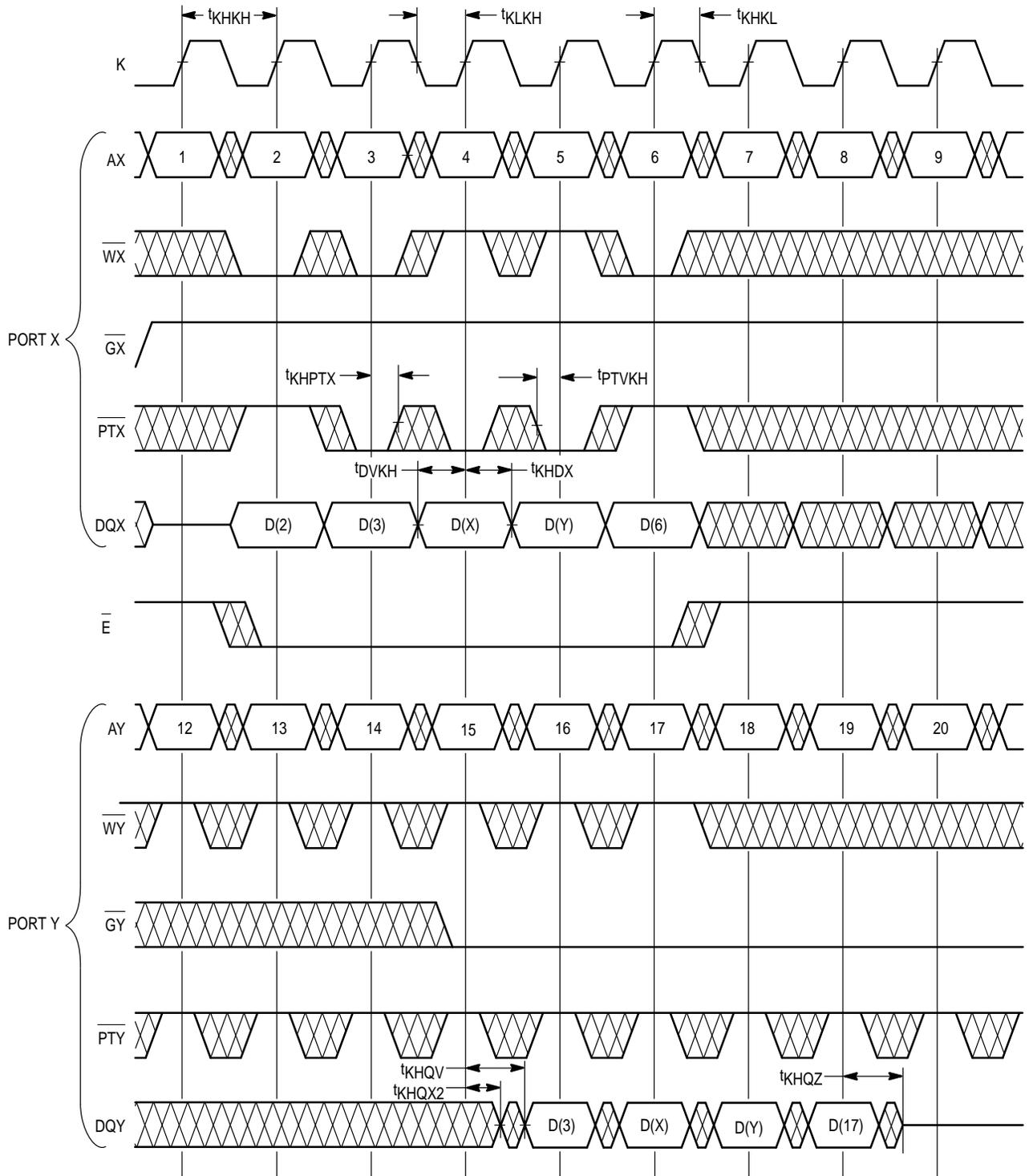
$\bar{E}$  Low =  $\bar{E}1$  Low and  $E2$  High.  $\bar{E}$  High =  $\bar{E}1$  High or  $E2$  Low.
