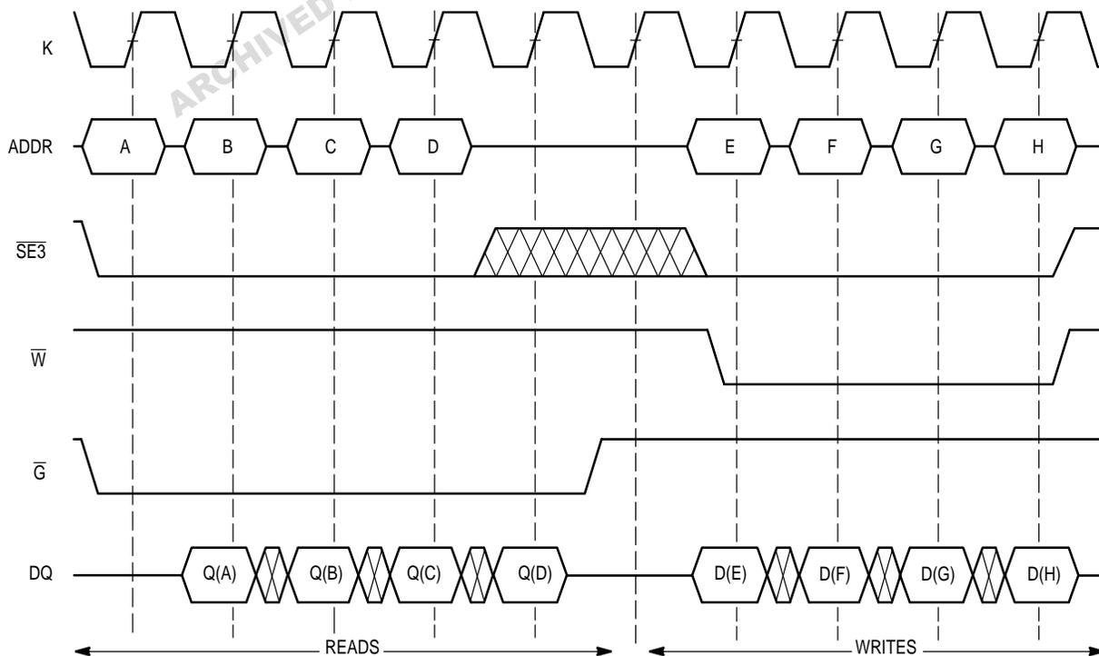
Figure 2. Example Configuration as Non-Burst Synchronous SRAM
