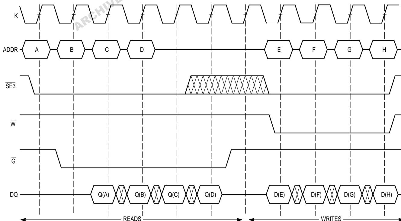
Figure 2. Example Configuration as Non-Burst Synchronous SRAM
