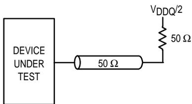
Figure 1. AC Test Load
