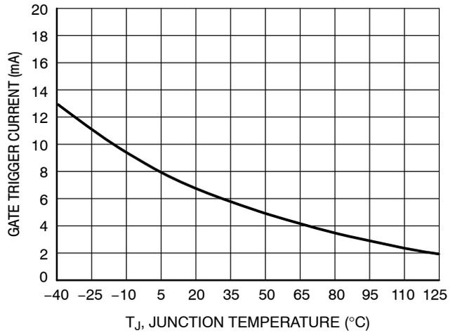
Figure 4. Typical Gate Trigger Current versus Junction Temperature
