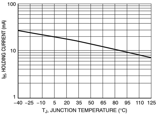
Figure 5. Typical Holding Current versus Junction Temperature
