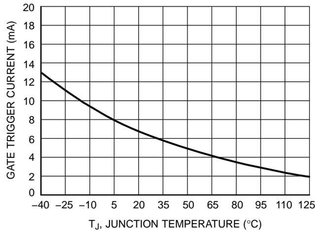
Figure 4. Typical Gate Trigger Current versus Junction Temperature
