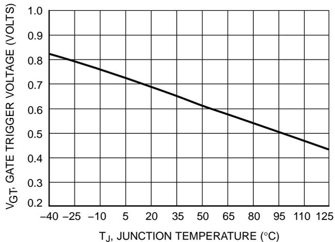
Figure 6. Typical Gate Trigger Voltage versus Junction Temperature
