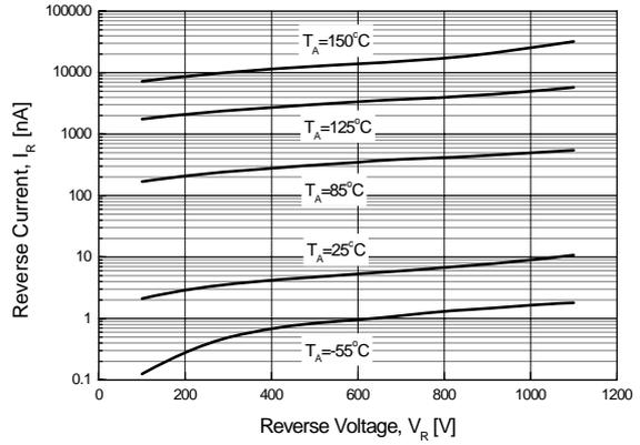
**Figure 2. Reverse Current vs Reverse Voltage (Per diode)**
