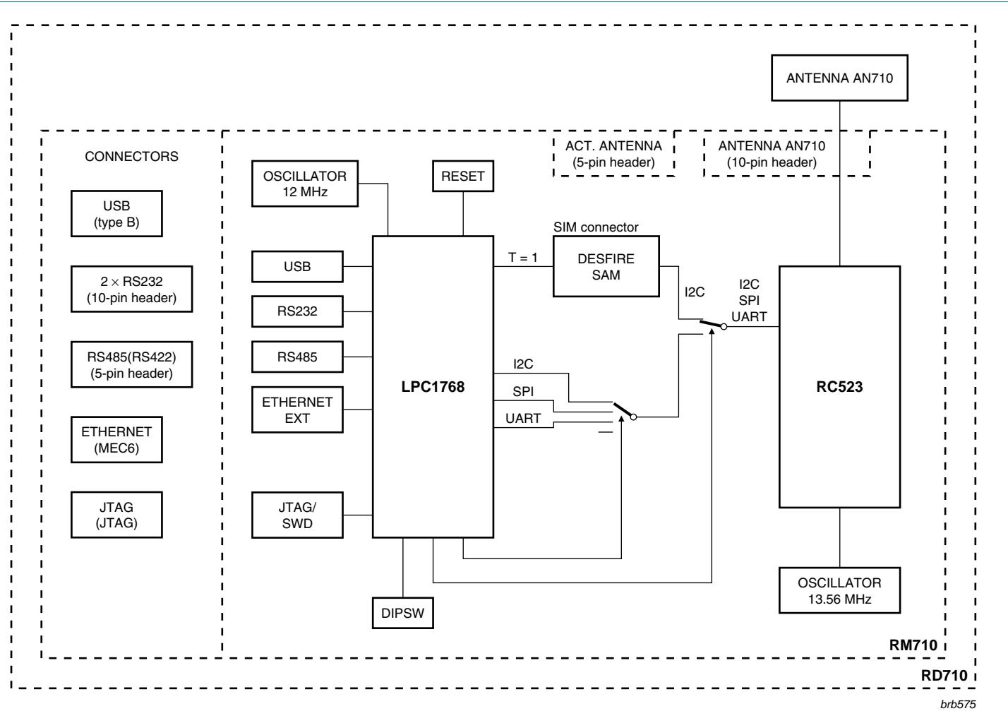
Fig 1. Block diagram RD710
