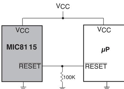
Figure 3.  $\overline{\text{RESET}}$  Valid to  $V_{CC} = 0\text{V}$ .
