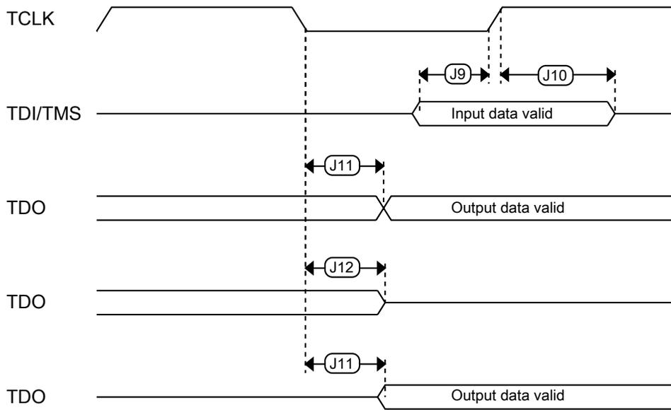
Figure 32. Test Access Port timing
