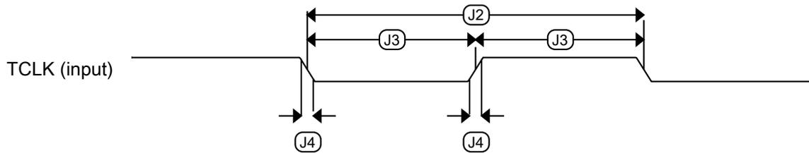
**Figure 30. Test clock input timing**
