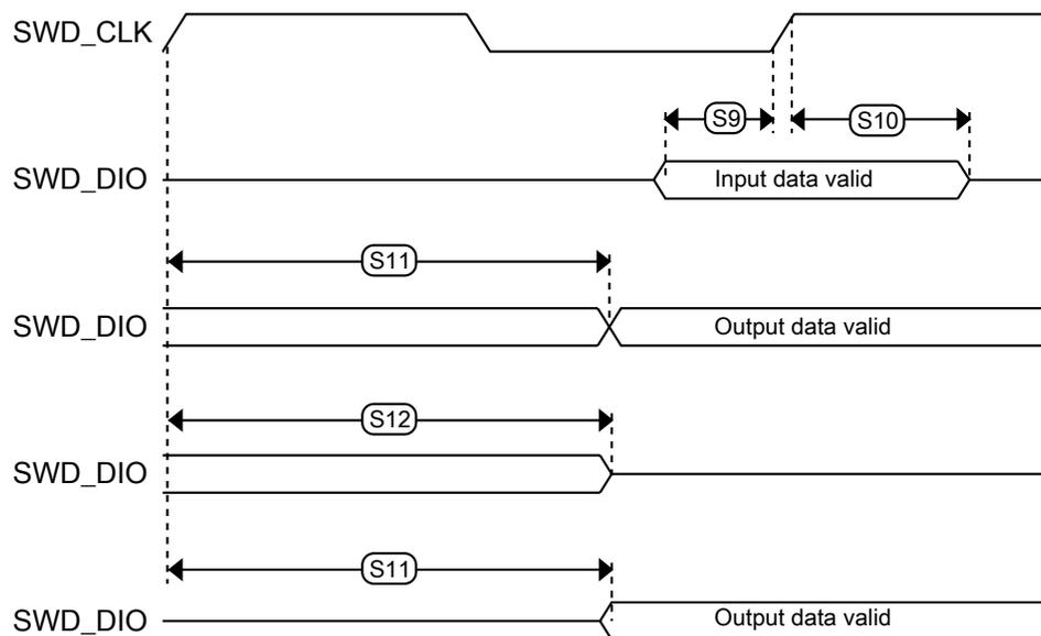
Figure 29. Serial wire data timing
