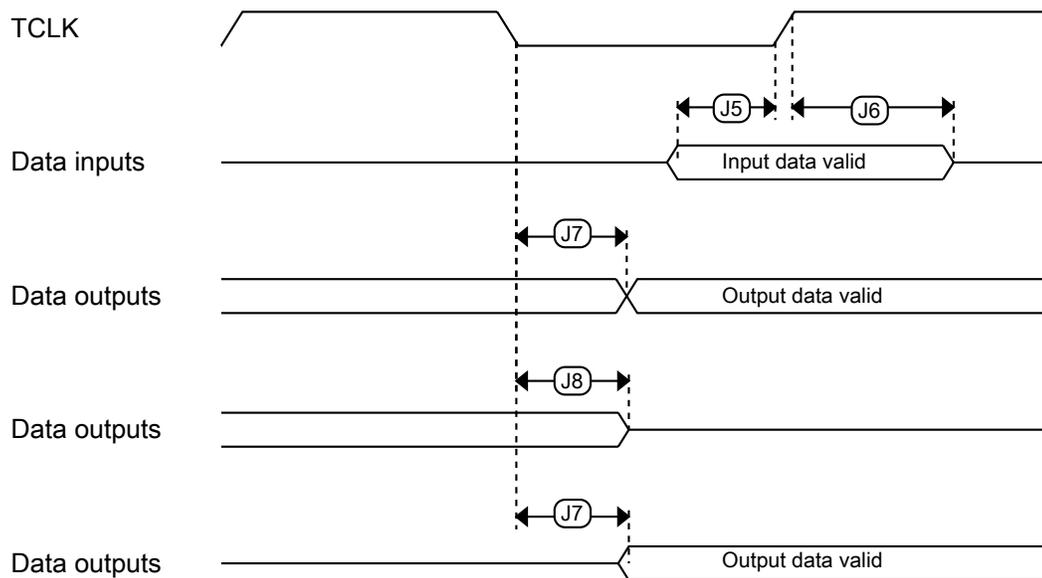
**Figure 31. Boundary scan (JTAG) timing**
