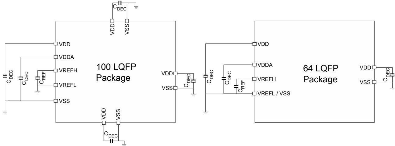
Figure 13. Pinout decoupling
