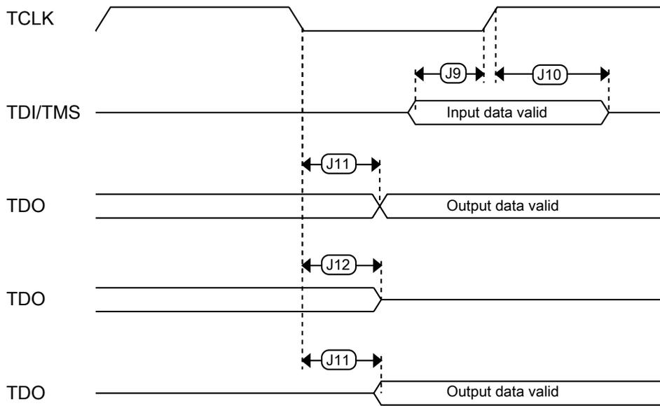
**Figure 32. Test Access Port timing**
