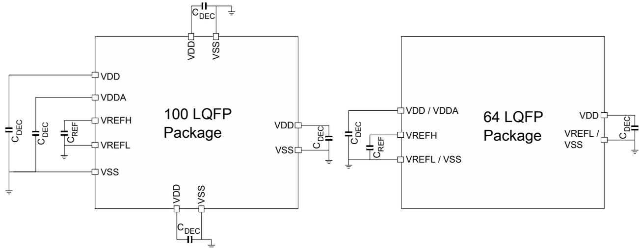
Figure 13. Pinout decoupling
