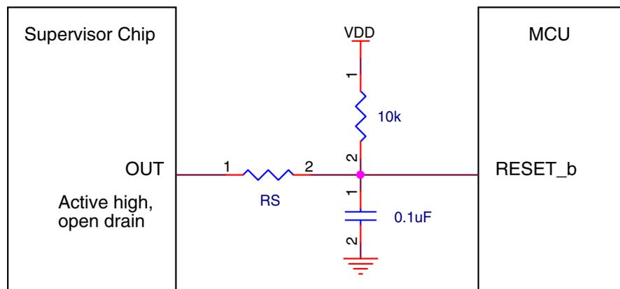
**Figure 37. Reset signal connection to external reset chip**
