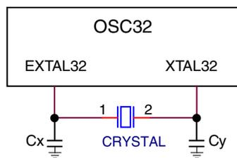
Figure 40. RTC Oscillator (OSC32) module connection – Diagram 1
