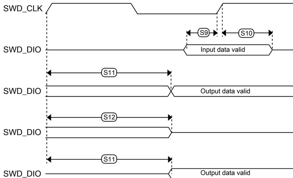
Figure 29. Serial wire data timing
