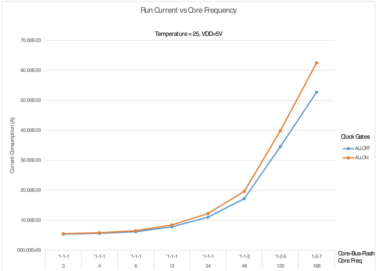
**Figure 14. Run mode supply current vs. core frequency**
