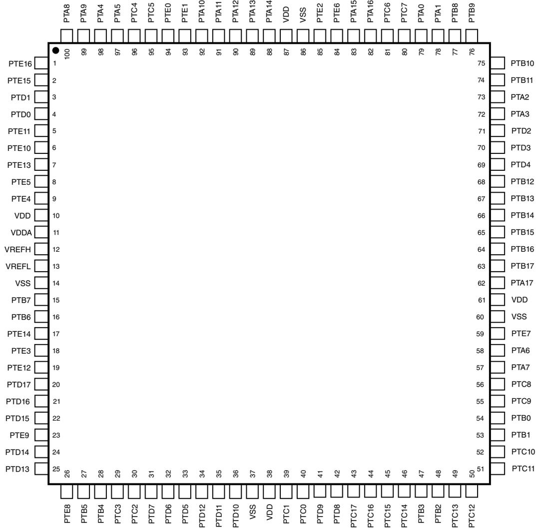
**Figure 7. 100 LQFP Pinout Diagram**
