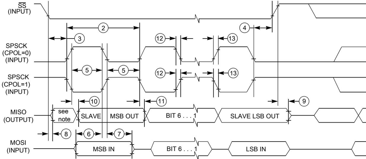
Figure 27. LPSPI slave mode timing (CPHA = 1)
