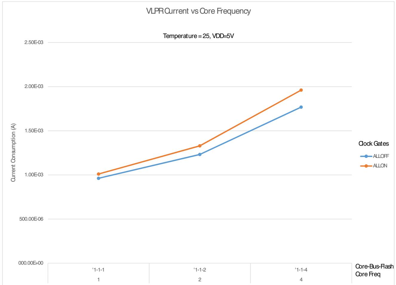
Figure 15. VLPR mode supply current vs. core frequency
