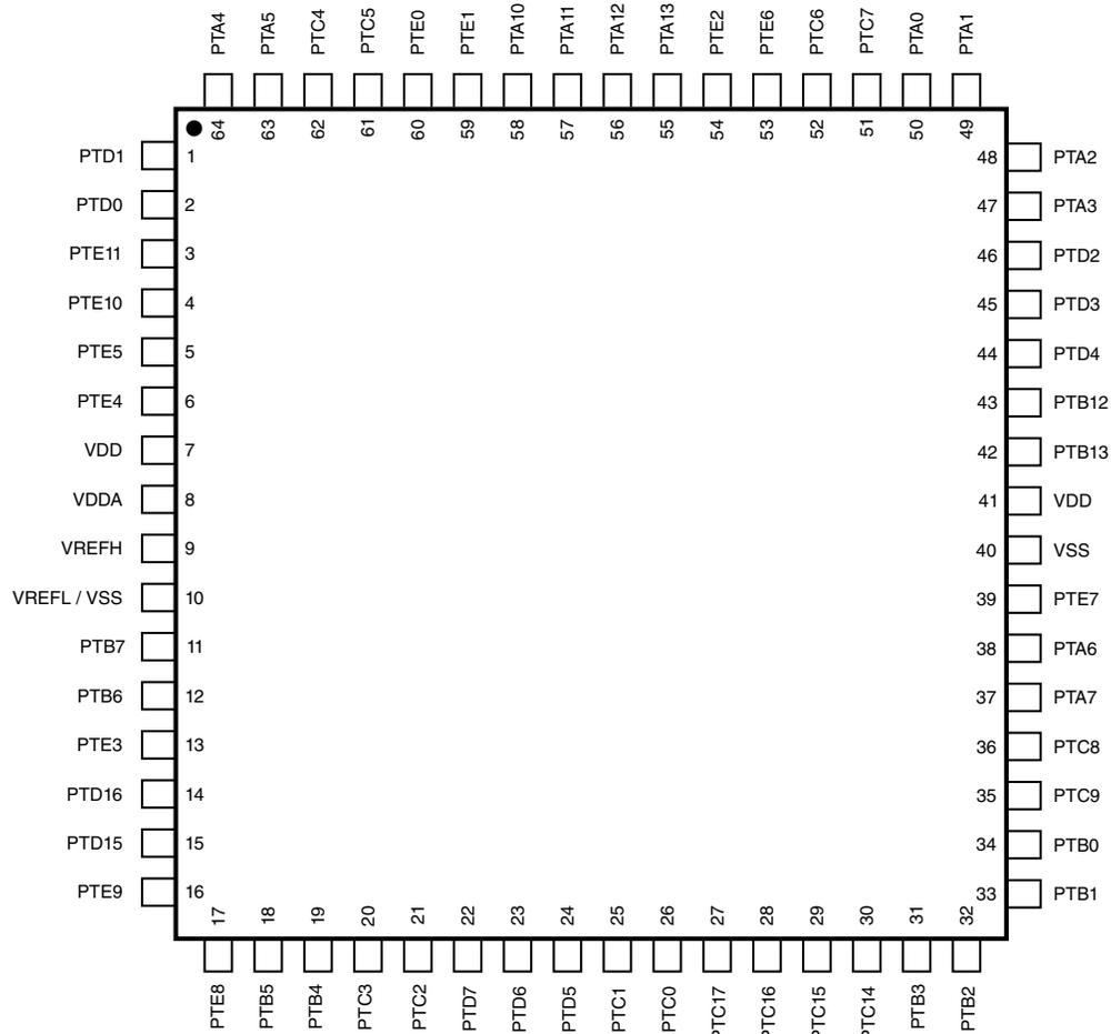
Figure 8. 64 LQFP Pinout Diagram
