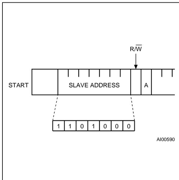
Figure 10. Write Mode Sequence
