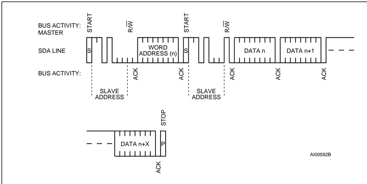
Figure 12. Alternate Read Mode Sequence
