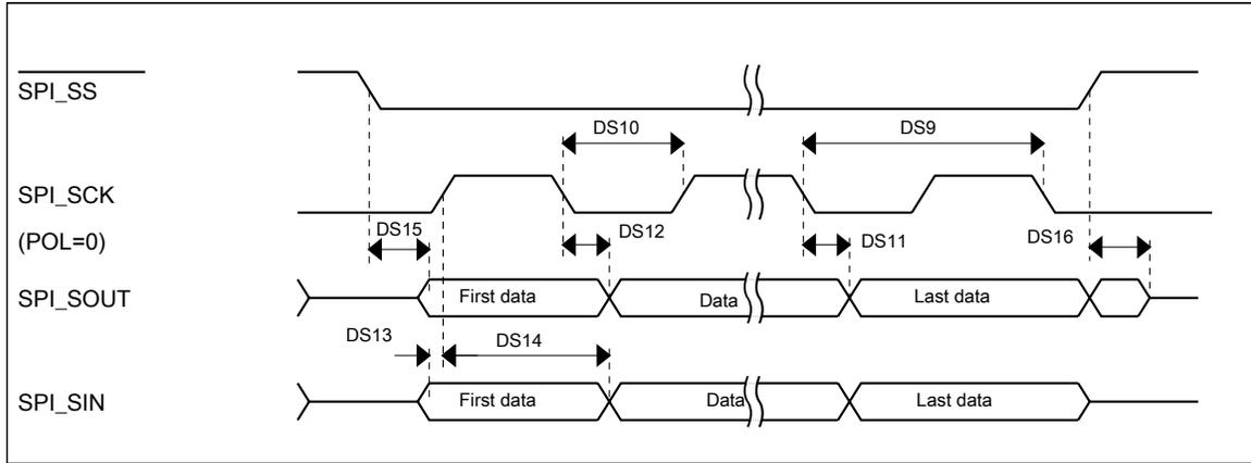
Figure 16. DSPI classic SPI timing — slave mode
