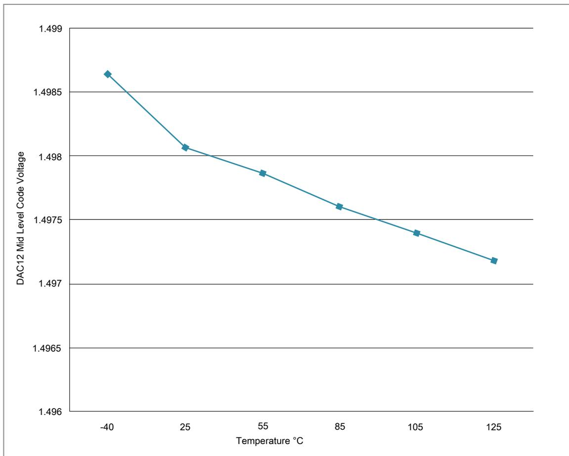
**Figure 12. Offset at half scale vs. temperature**
