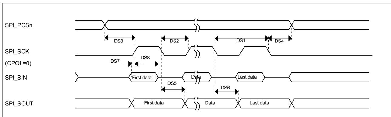
**Figure 13. DSPI classic SPI timing — master mode**
