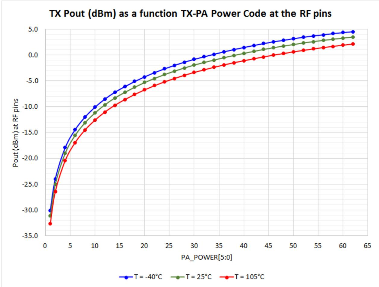
**Table 8. Transmit Output Power as a function of PA\_POWER[5:0]**
