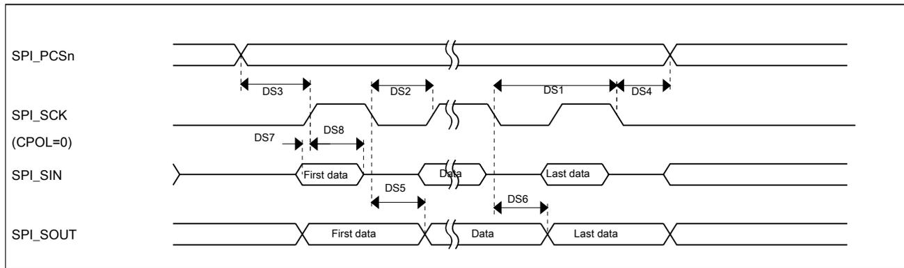
**Figure 15. DSPI classic SPI timing — master mode**
