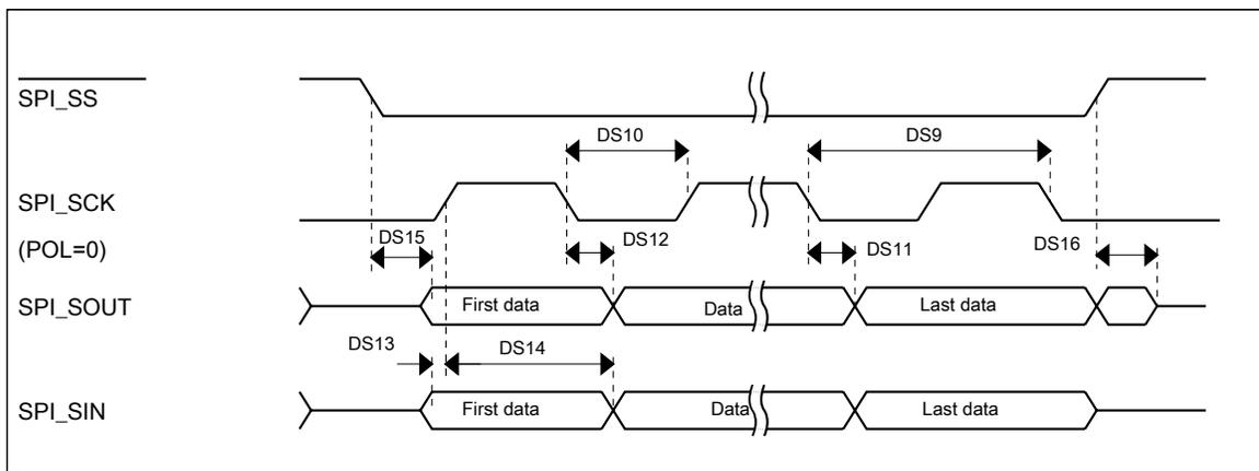
**Figure 14. DSPI classic SPI timing — slave mode**
