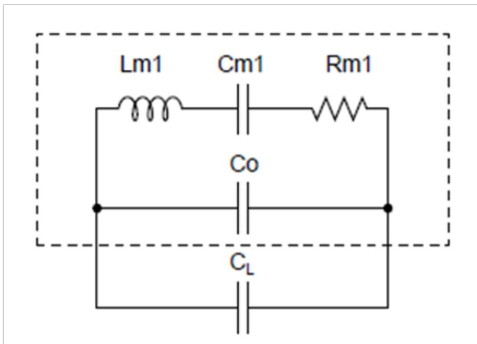
Figure 7. Crystal Electrical Block Diagram
