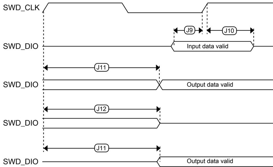
Figure 6. Serial wire data timing
