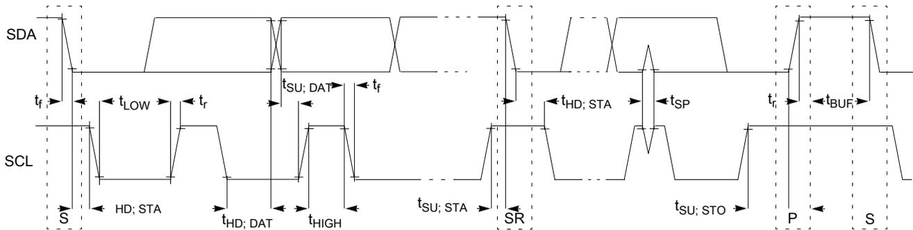
Figure 17. Timing definition for fast and standard mode devices on the I<sup>2</sup>C bus
