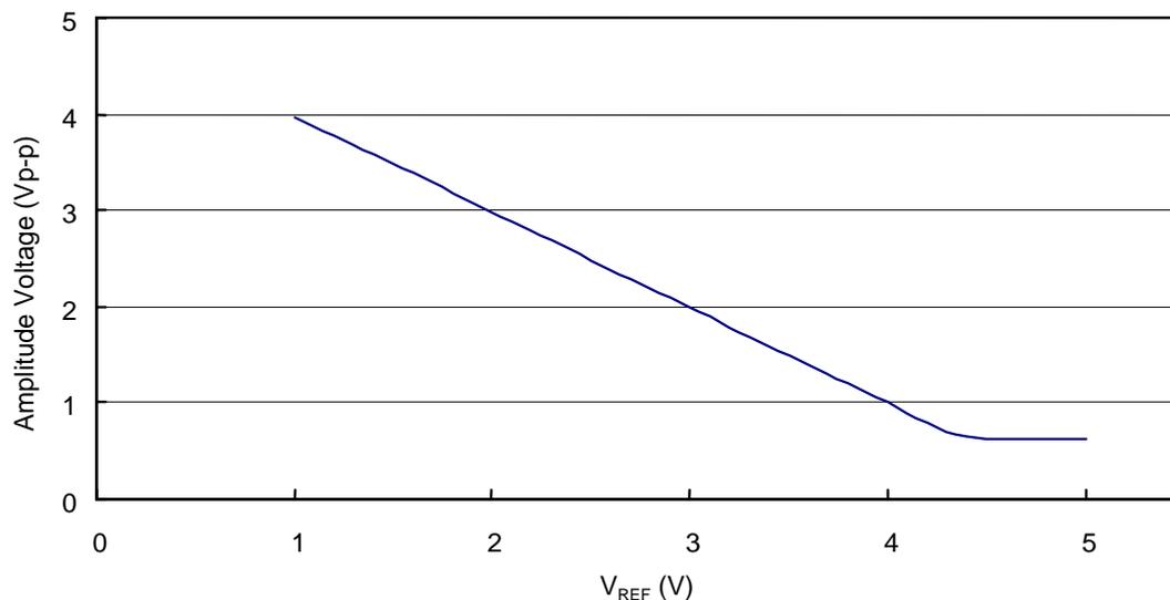
**Figure 7.1  $V_{REF}$  – AOUT Amplitude**
