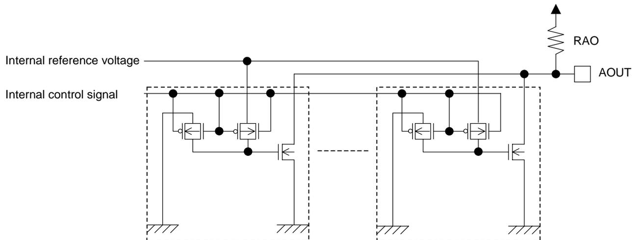
As shown above, the ML2215 uses current type DACs.
