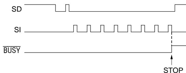
**Figure 6.1 Timing for Stop Code Input - 2-pin Interfacing**
