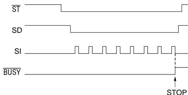
**Figure 6.2 Timing for Stop Code Input - 3-pin Interfacing**
