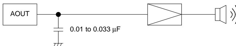
The capacitor is used for improving a voice quality. Check the voice quality before determining the capacitor value. If the voice quality is excellent without connecting a capacitor, no capacitor is required.
