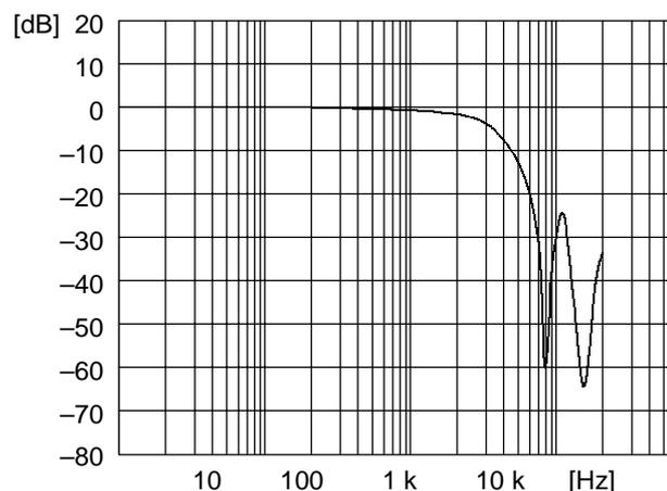
Figure 10.1 LPF Frequency Characteristics ( $f_{\text{SAM}} = 8 \text{ kHz}$ )
