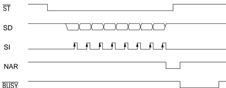
Figure 4.3 Timing Chart of Serial Input
