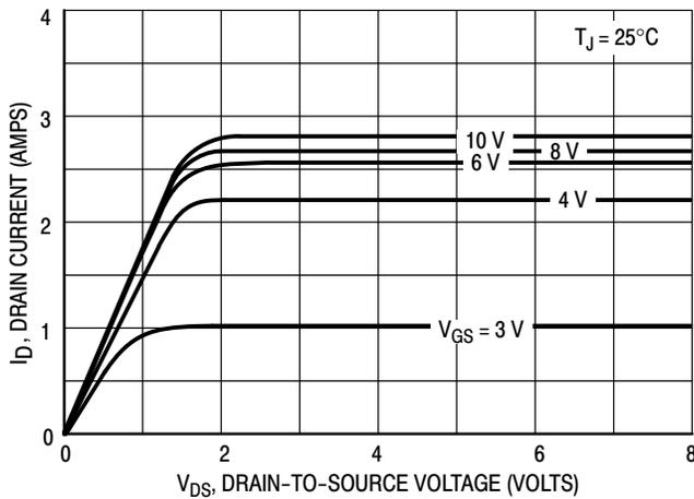
Figure 1. Output Characteristics
