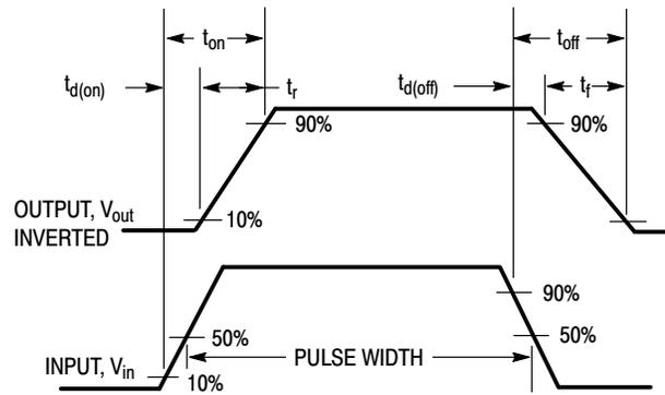
Figure 11. Switching Waveforms
