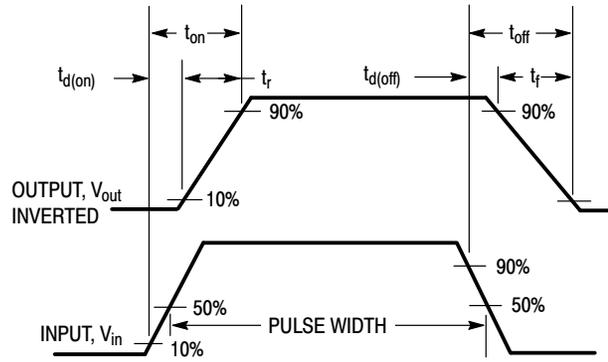
Figure 11. Switching Waveforms
