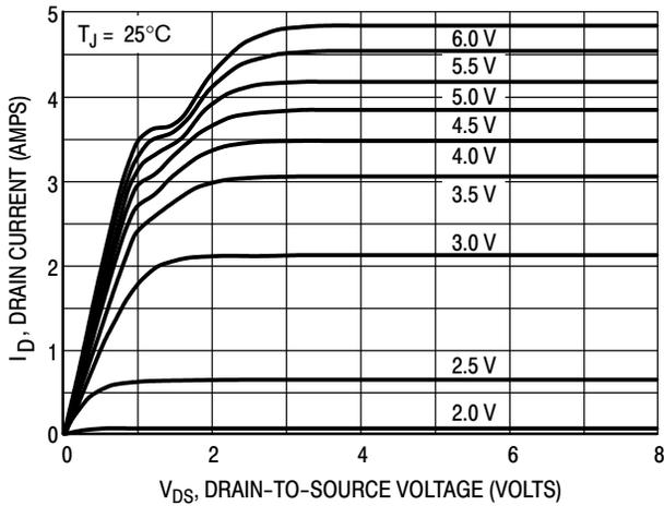
Figure 1. Output Characteristics
