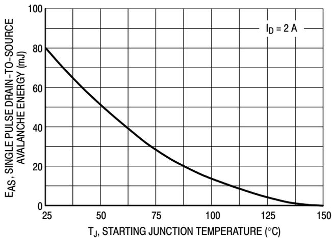
**Figure 6. Maximum Avalanche Energy versus Junction Temperature**
