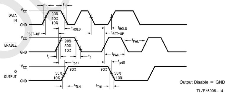
**MM54C373/MM74C373 TRI-STATE Octal D-Type Latch**
