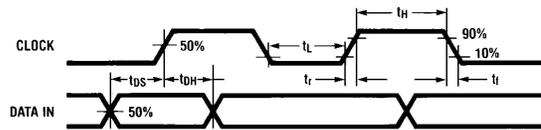
For the purposes of AC measurement,  $V_{IH} = 2.4V$ ,  $V_{IL} = 0.8V$ .
